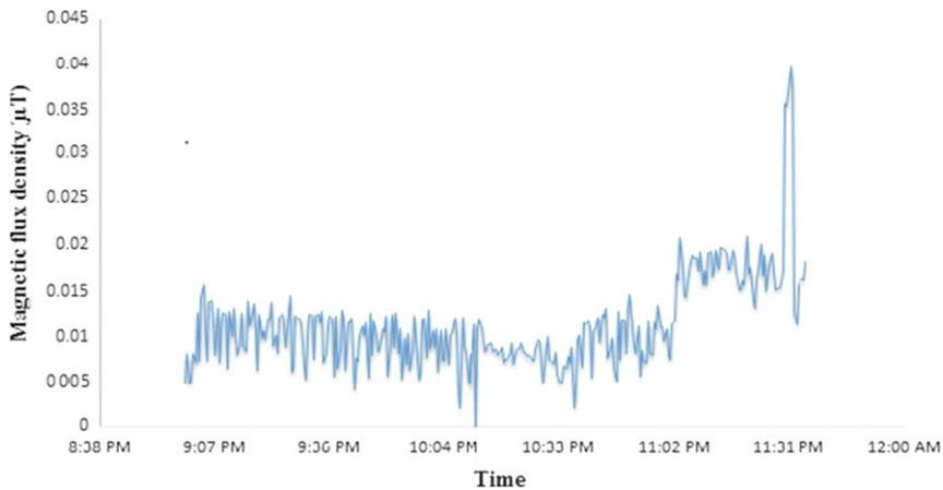
Figure 2. Variations of ELF magnetic flux densities over 2.5 h period, and one meter above ground level at residence R10.
