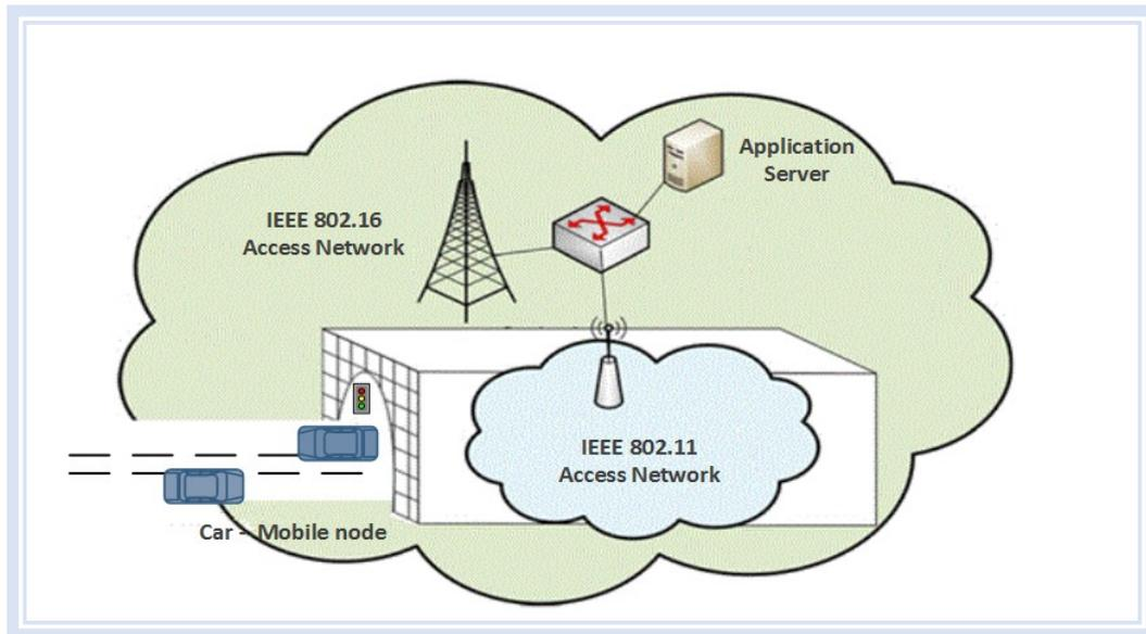
Figure 2.1: Example of wireless access networks of IEEE 802 family [AAMH11].
