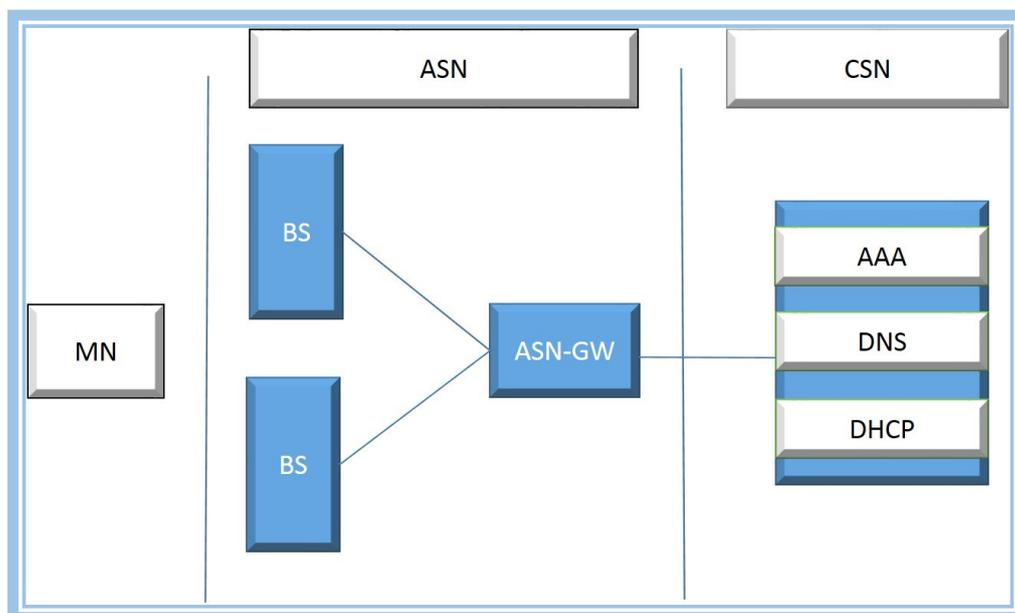
Figure 2.2: WiMAX architecture [TT10].
