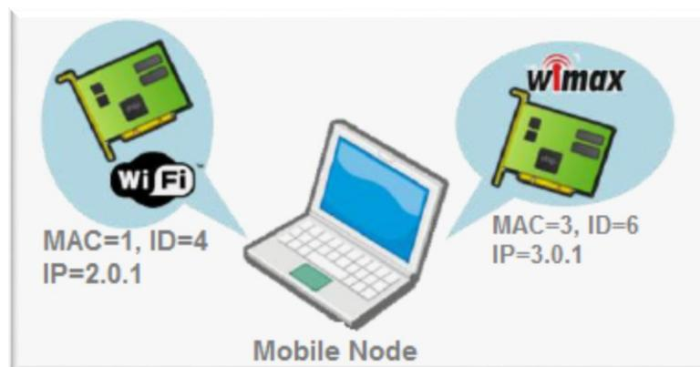
Figure 2.5: Mobile node with multiples interfaces [AAQ10].
