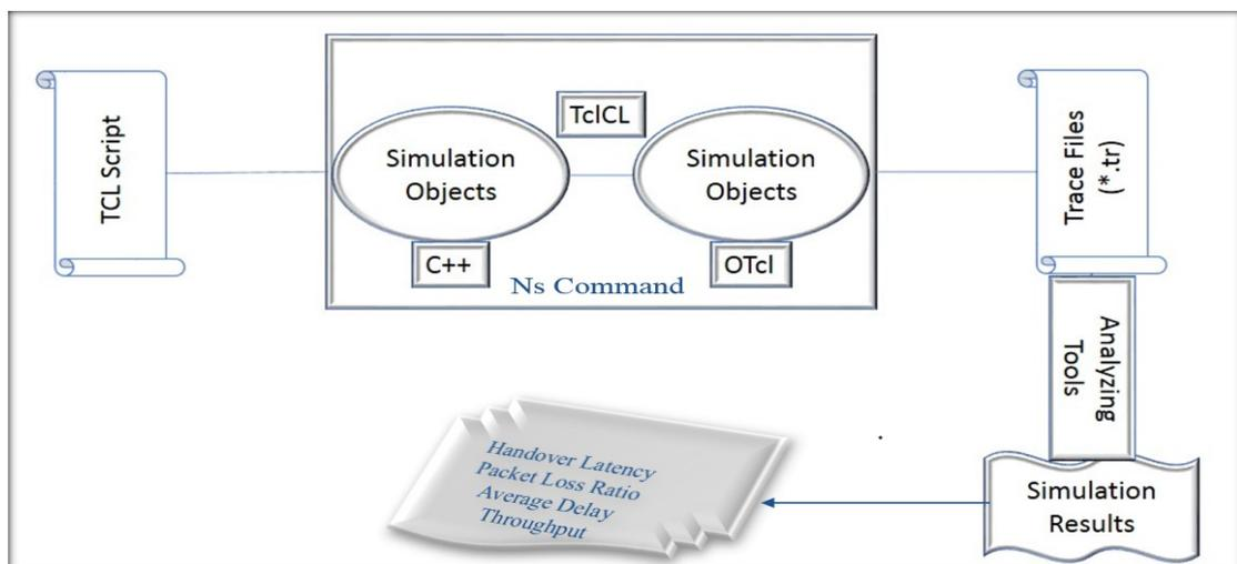
Figure 3.2: NS-2 architecture and simulation process.
