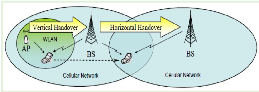
Figure 2.4: Horizontal and Vertical handover [Yan10].
