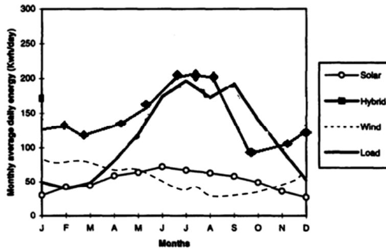
Figure 11. Monthly distribution of solar, wind, and hybrid power in Gaza city at 50 m height (hybrid systems consisting of 3 kW WECS and 25 m<sup>2</sup> of photovoltaic solar) [27].
