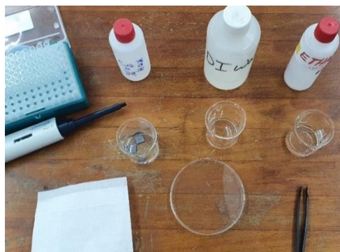
Fig. (3.2): Chemicals used for etching, Ethanol, DW and KOH(30% wt)
