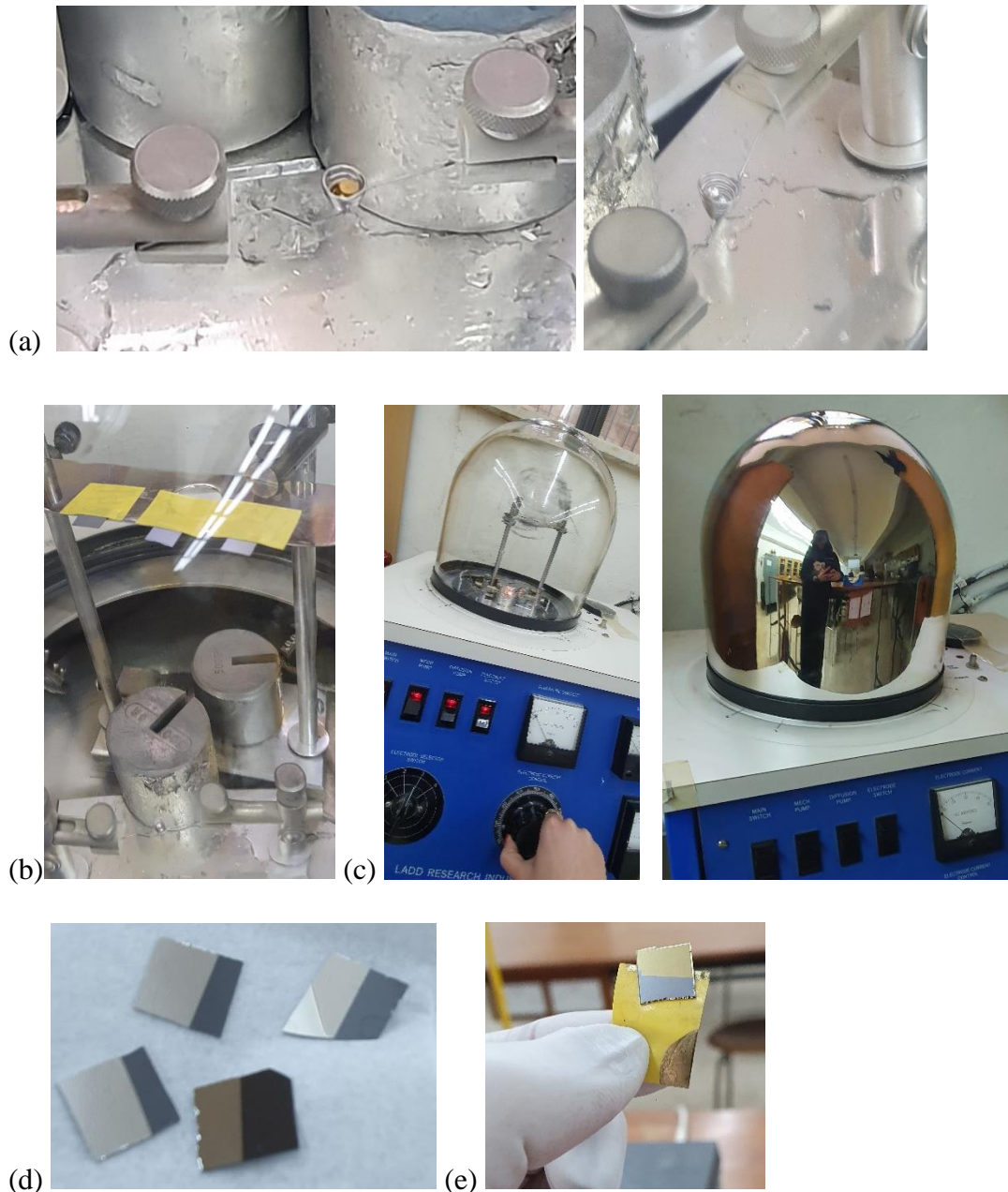
Fig. (3.10): (a) the Gold and Metal placed in the crucible. (b) the Si samples fixed at the sample holder. (c) Slowly allowing the current to pass through and cause the heating up of the metal for evaporation (d) the resulted Ag\NPs\Si Schottky diode. (e) the resulted Au\NPs\Si Schottky diode.
