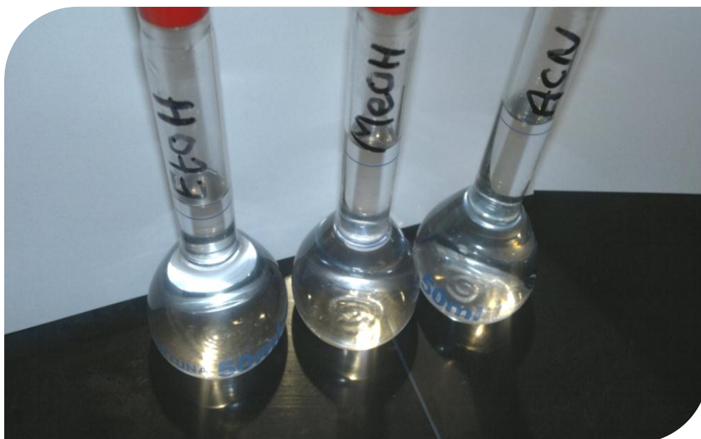
Figure 30 Photos for sample representing co-crystal obtained from each co-solvent used in water, after sonication for 15 minutes. It is completely dissolved
