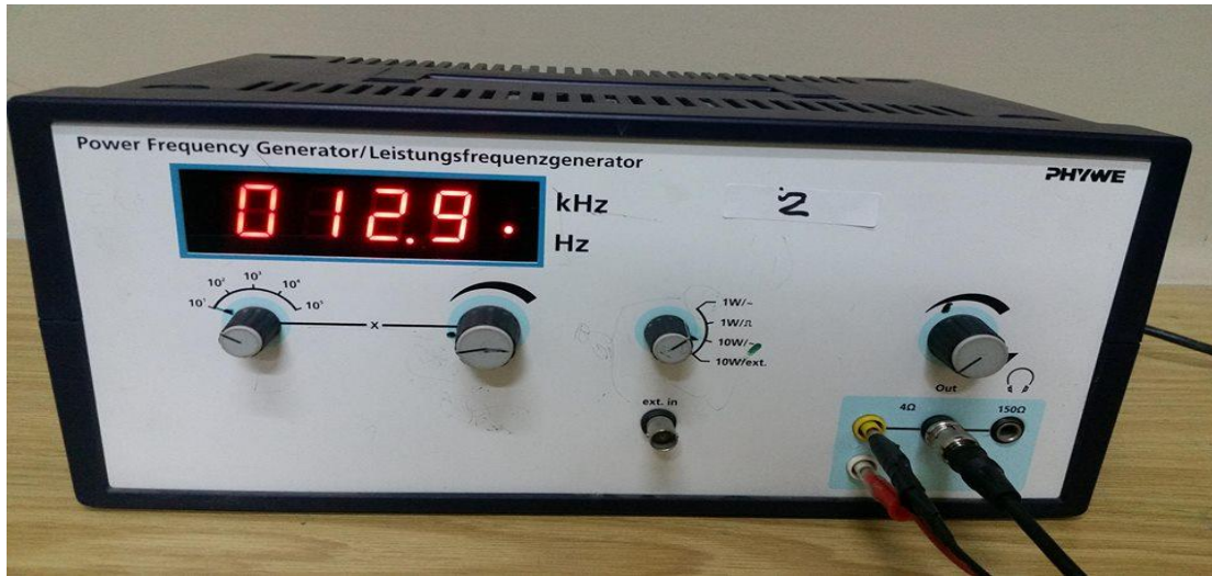
Figure 3.3: Photo of Power frequency generator.
