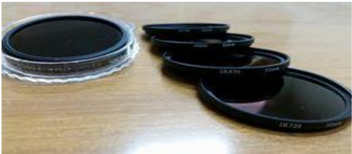
Figure 3.2: Photo of IR filters in different wave length (1000 nm, 950 nm, 850 nm, 760nm and 720nm).
