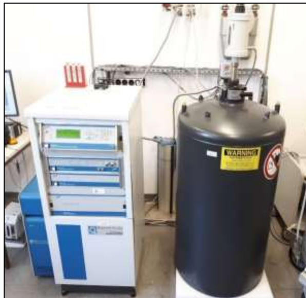
Figure 4.9: The Physical Property Measurement System used for the measurement of macroscopic magnetization data.
