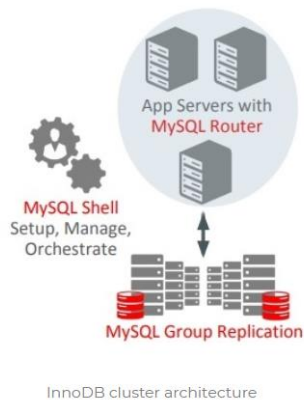
Figure 2.6: InnoDB cluster architecture [22]
