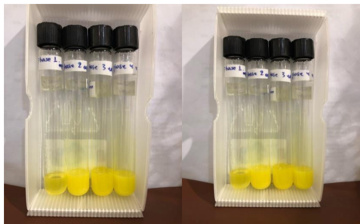
Figure. 12. Turbid yellow solutions with precipitate, when we added 5 mg of Tenoxicam to the 0.8% (0.04g/5g microemulsion).
