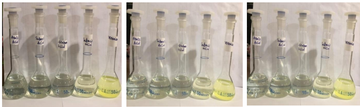
Figure. 20. The clarity of solubility of 5 mg of co-crystal/ 40 ml of water, compared to 5 mg of solubility of Tenoxicam / 40ml of water.
