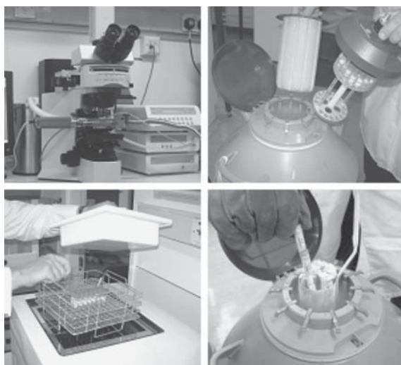
Figure 21.3 Examples of cryotechnologies, equipment for cryopreservation and cryopreservation protocol development. Top left: cryomicroscope; top right: cryostat with vapour phase cooling device; bottom left: programmable freezer; bottom right: cryopreserved cells stored on cryorods in a vapour phase LN Dewar. (Photographs by kind permission of N.I.B.S.C.).
