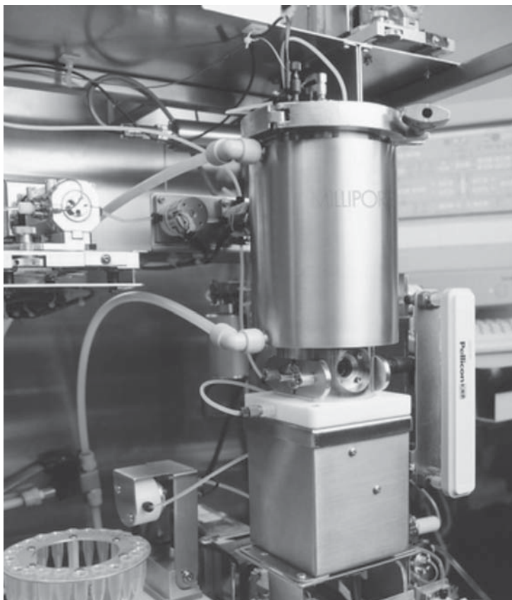
Figure 17.4 Automated Process Development System (APDS) manufactured by Millipore Corporation for small-scale ultrafiltration studies. (Reproduced by permission of Millipore Corporation.)
