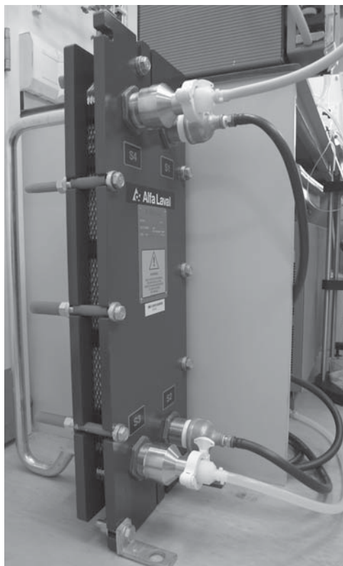
Figure 18.5 A 1/10-scale heat exchanger used in the development of a process to cool 50L of clarified harvest in the production of a live virus vaccine. Photo courtesy of Jim Mills, reproduced with permission of Xenova.
