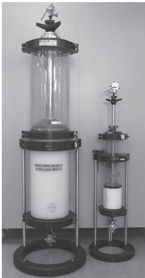
Figure 18.3 Pilot-scale columns used in Phase II clinical manufacture. A 30-litre size exclusion column and a 2-litre ion exchange column used for production of clinical lots for a protein vaccine product at Xenova. In these Millipore Vantage A columns, the headspace above the top adjustable adapter can be pressurised to enable rapid and consistent column packing. Photo courtesy of Jim Mills, reproduced with permission of Xenova.
