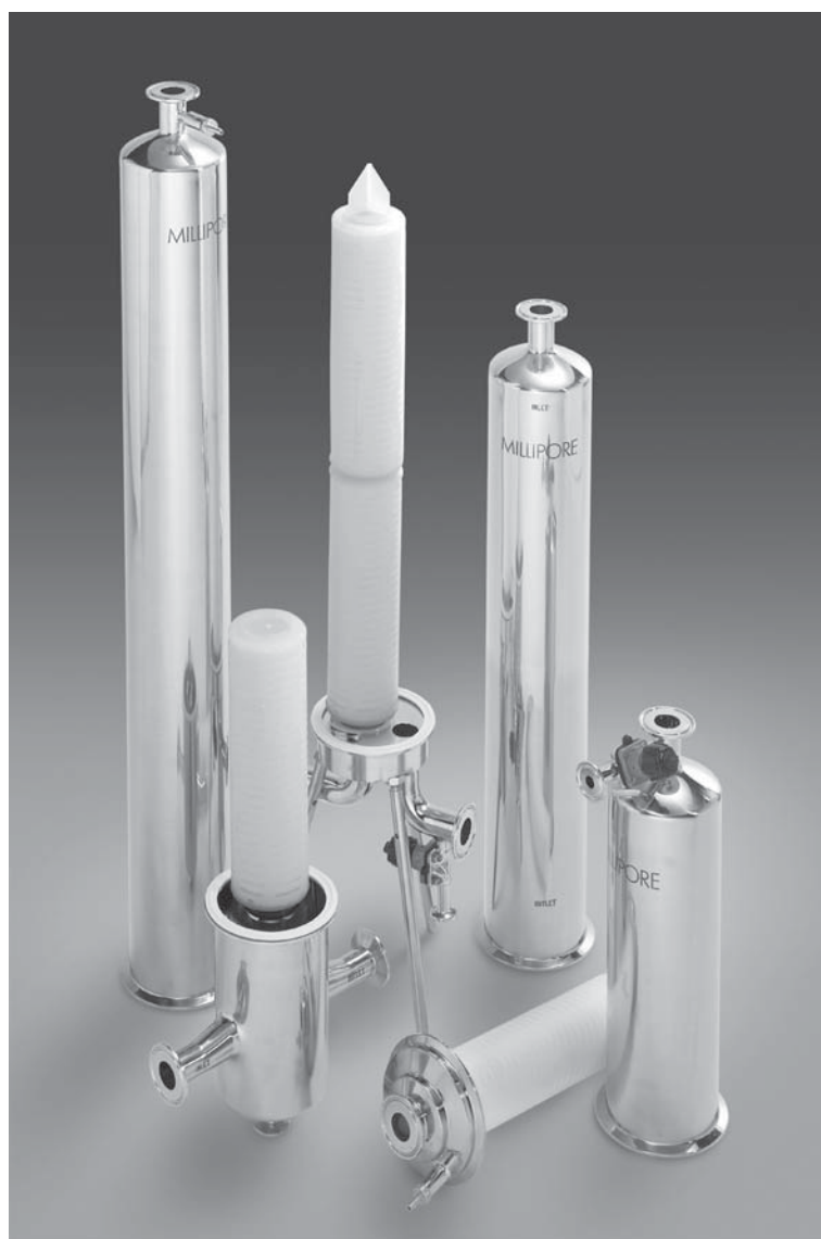
Figure 14.2 Filter cartridges and housings for sterilization of gases and liquids. From left to right: 10" cartridge for gases with a collector for condensates; 20" cartridge for liquids (e.g. culture media); 10" cartridge for utilities (e.g. WFI), to be mounted horizontally in line (courtesy of Millipore).
