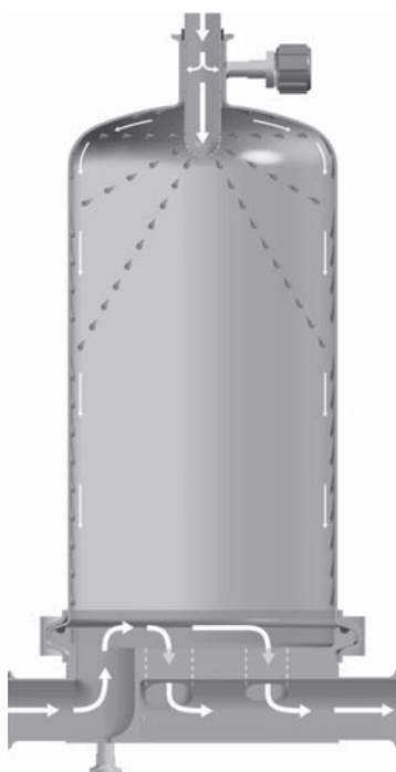
Figure 14.9 CIP of a filter housing. The housing is cleaned by the simultaneous circulation of solutions through a spray ball at the top and through the inlet and outlet process piping (reproduced with permission from Graf and Bernsley 2002).
