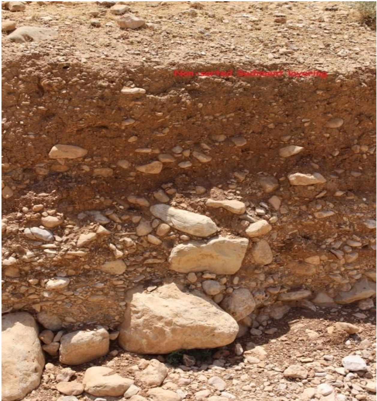
Figure 4.5: non-sorted sediment, it often formed when stream velocity suddenly decreases. It's mixed in size, shape, and density. Photo was captured by Soil and Hydrology lab/ Al-Quds university
