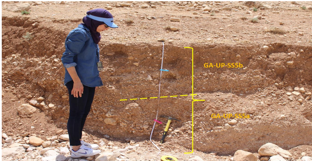
Figure 4.13: GA-UP-SS5 sample in 2018 it is possible to notice the rise in the layers that occurred, as it only increased one thick layer within a year. Photo was captured by Soil and Hydrology lab/ Al-Quds university
