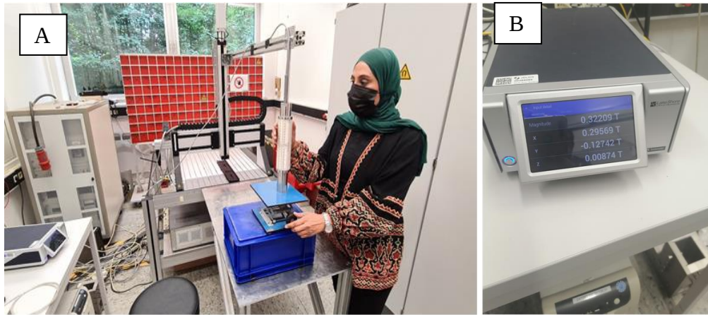
Figure 3.23: Measure the magnet flux density inside the inner magnet Mandhala
