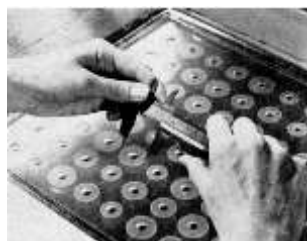
Figure 12: Measuring the diameter of zones using vernier scale calipers.
