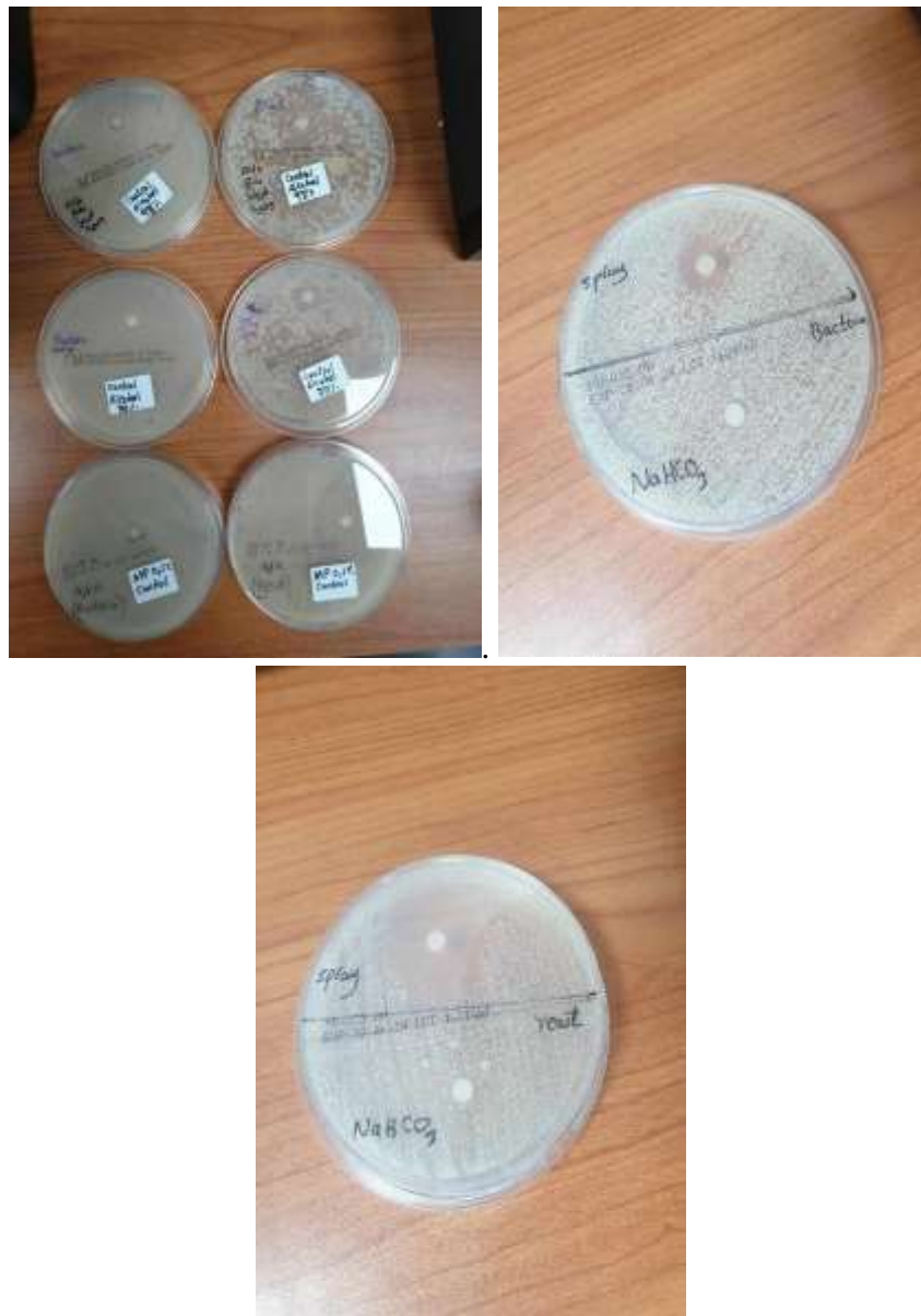
Figure33: zone of inhibition by 98%, 70% alcohol, 0. 1% methyl paraben, and 0.8% NaHCO 3 on yeast and bacteria
