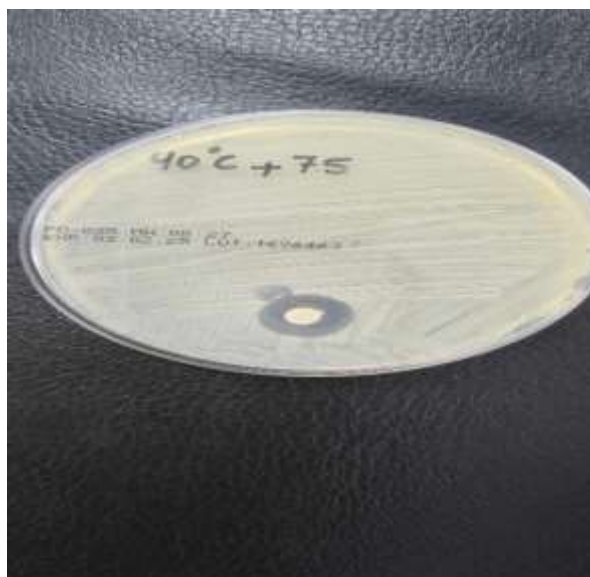
Figure 36: Diameter zone of inhibition on bacteria after incubation for 2 months under 40^{\circ}\text{C} \pm 2^{\circ}\text{C}/75\% \text{RH} \pm 5\% \text{RH}
