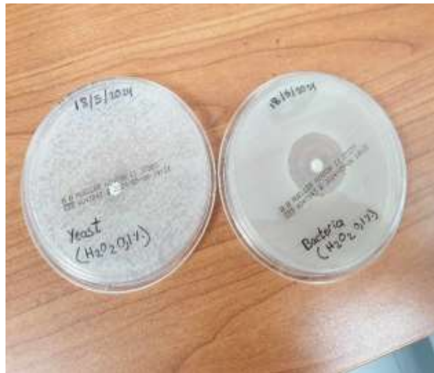
Figure 9: Zone of inhibition of H 2 O 2 on yeast and bacteria at concentrations of 0.1%
