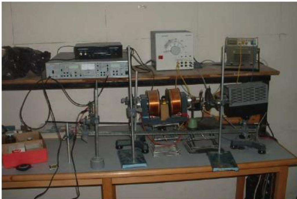
Fig. 3. The complete setup used to study Faraday effect of some vegetable oils
