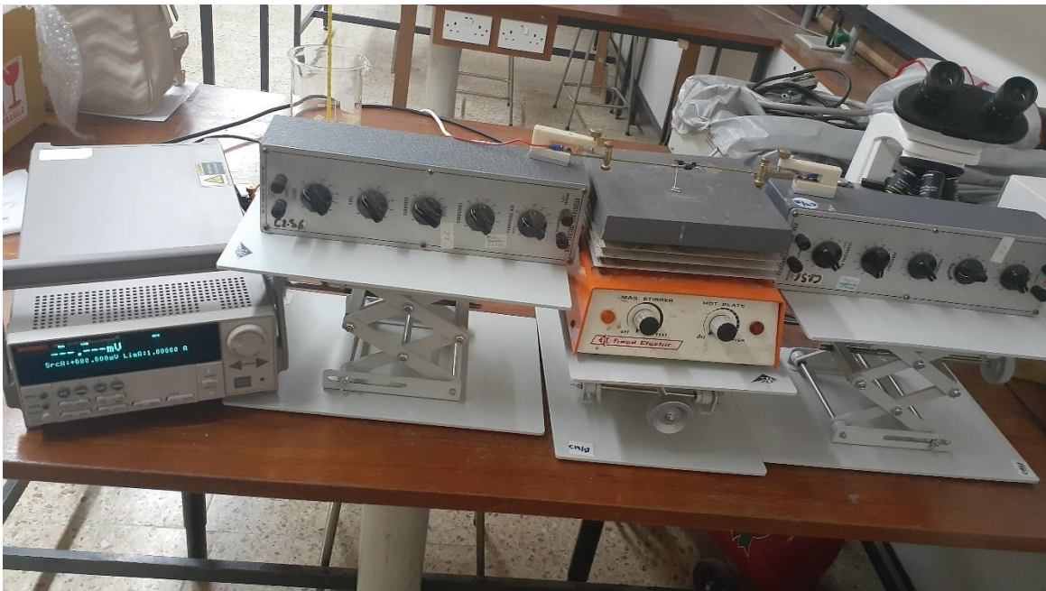
Figure 3.12: set up for IV-Characteristics.
