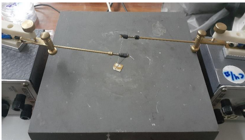
Figure 3.13: during taking the IV-measurements for a sample.
