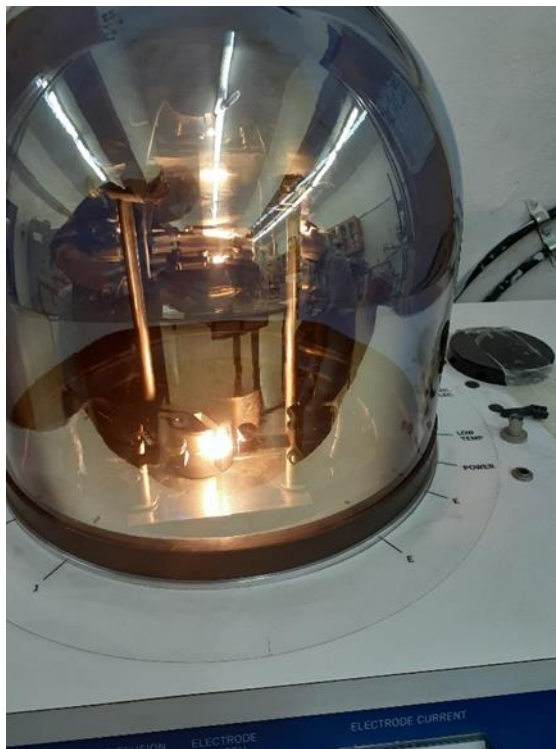
Figure 3.11: the thermal evaporator during metal deposition process.
