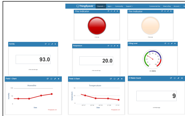
Fig. 4. ThingSpeak Dashboard showing various monitored data, such as e-waste count, filling level, fire indicator, temperature, and humidity.
