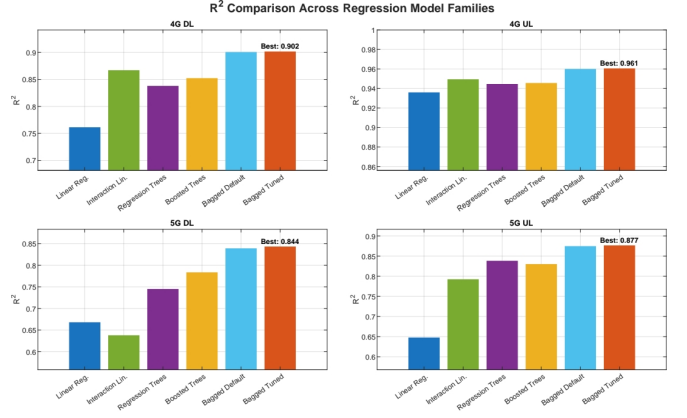
Fig. 5. Coefficient of determination comparison across regression model families for 4G and 5G downlink/uplink throughput prediction.
