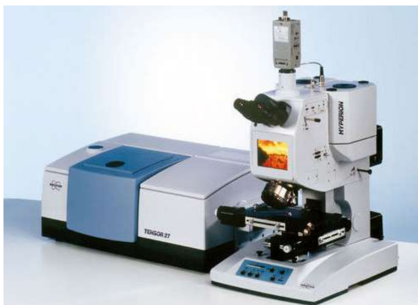
Figure 3.4: FTIR imaging system containing a FTIR microscope (Hyperion 3000, Bruker Optics) with FTIR spectrophotometer (Tensor 27, Bruker Optics) [104].
