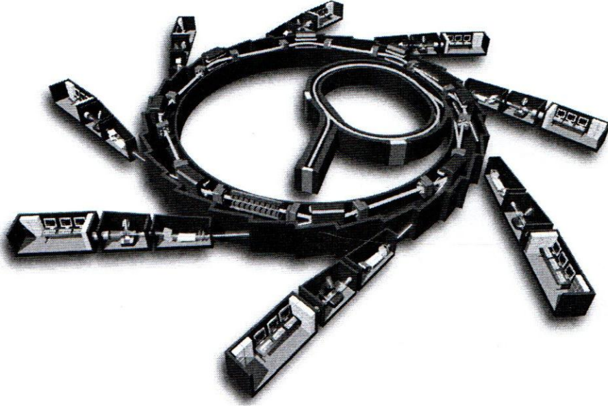
Figure 1.2 The layout of atypical synchrotron, showing a pre-injector, booster, storage ring, and beamlines (www.soleil.fr)
