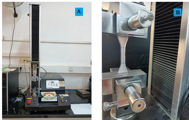
Figure (3.16): A: Universal testing machine of polymer (tensile test) B: Tensile specimens during testing.
