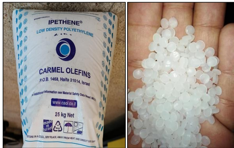
Figure (3.2): LDPE pellets obtained from the Materials Engineering faculty, Al-Quds University.
