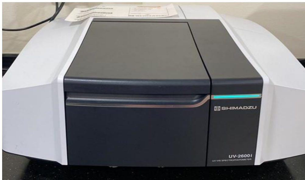
Figure 3.2.2 UV-visible (Shimadzu UV-2600i) spectrophotometer instrument (Equip at Palestine Technical University Kadoorie, Nanotechnology research lab).
