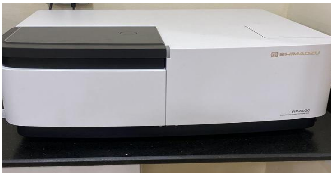
Figure 3.2.3 Photoluminescence (SHIMADZU RF6000) spectroscopy instrument. (Equip at Palestine Technical University Kadoorie, Nanotechnology research lab).
