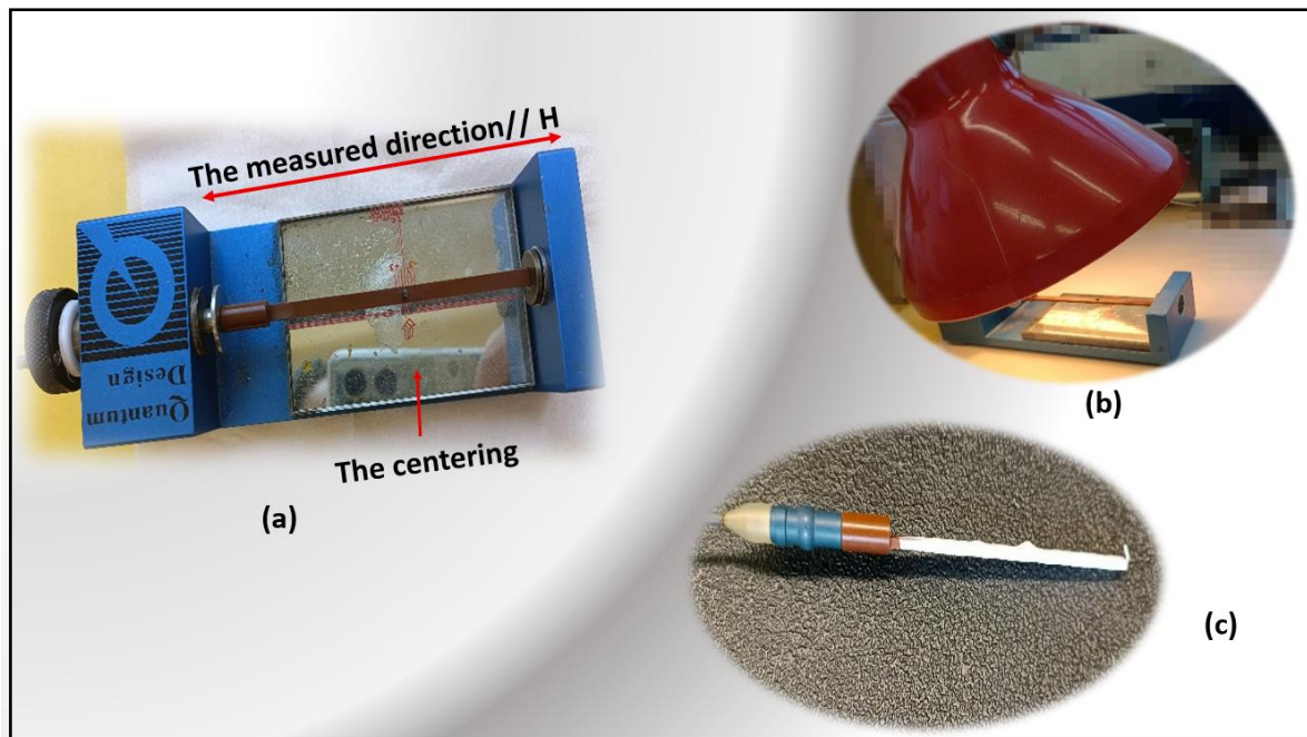
Figure 3.9: The sample preparation procedure. (a) Centering the sample on its holder using the mounting station (b) the sample under light to be dried (c) rapping the sample by Teflon.
