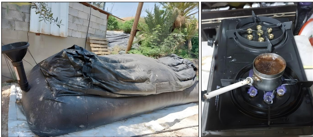
Figure 3.6: Home biogas system ready to work with the first production of gas.
