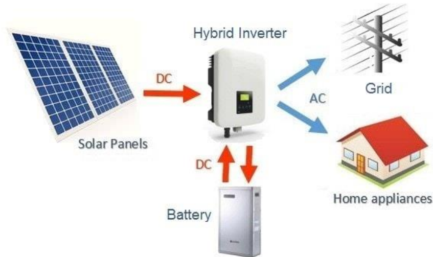
Figure 2.3: Solar Hybrid PV System (Nuetech Solar, n.d.).
