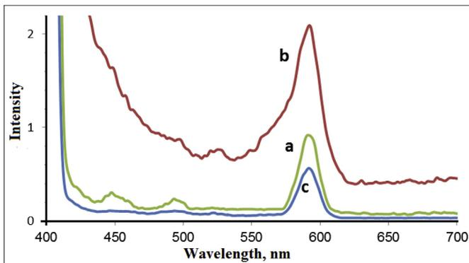
Fig. 3. Photoluminescence spectra for CBD of CuSe thin films, deposited by different techniques, a) CBD/ECD, b) CBD, and c) ECD.
