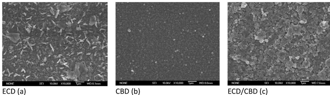
Fig. 4. SEM micrographs for CuSe films prepared by different methods, (a) ECD, (b) CBD and (c) ECD/CBD.
