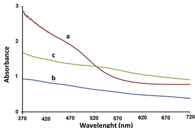
Fig. 1. Electronic absorption spectra for CBD of the CuSe thin films, deposited in different techniques, a) CBD/ECD, b) CBD and c) ECD.
