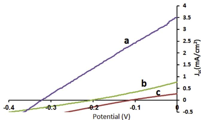
Fig. 8. Photo  $J$ - $V$  plots measured for different CuSe film preparations: (a) ECD/CBD, (b) CBD and (c) ECD. All measurement were made at room temperature using  $[\text{Fe}(\text{CN})_6]^{4-}/\text{Fe}(\text{CN})_6^{3-}$  redox couple, vs. NHE.
