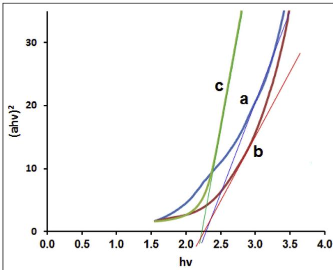
Fig. 2. Tauc plots for CuSe films prepared by different methods assuming a direct band gap. a) ECD b) CBD c) ECD/CBD.
