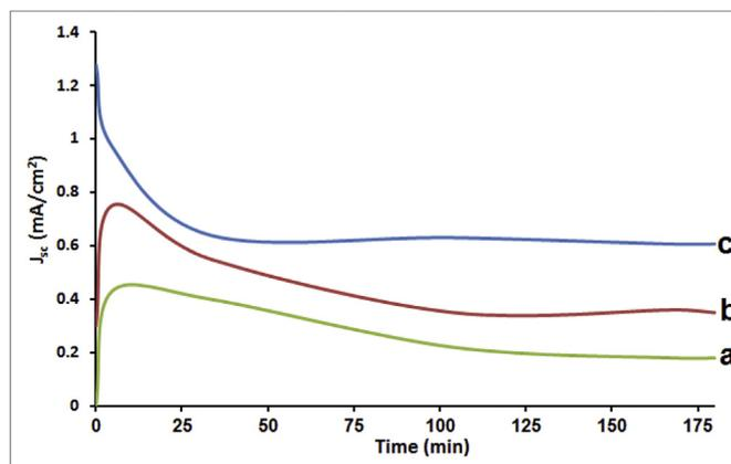
**Fig. 10.** Film electrode stability, showing plots of *J<sub>SC</sub>* value vs. time for different CuSe film preparations: (a) ECD, (b) CBD and (c) ECD/CBD. All measurement were made at room temperature using [Fe(CN)<sub>6</sub>]<sup>4-</sup>/[Fe(CN)<sub>6</sub>]<sup>3-</sup> redox couple, vs. NHE.
