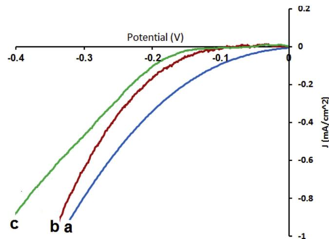
Fig. 7. Dark  $J$ - $V$  plots for different CuSe film preparations: (a) ECD, (b) CBD and (c) ECD/CBD. All measurement were made at room temperature using  $[\text{Fe}(\text{CN})_6]^{4-}/\text{Fe}(\text{CN})_6^{3-}$  redox couple, vs. NHE.
