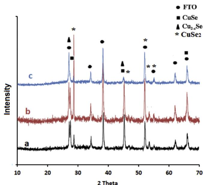
**Fig. 9.** XRD patterns measured for ECD/CBD-CuSe films: (a) annealed and quickly cooled (b) annealed and slowly cooled and (c) non-annealed.
