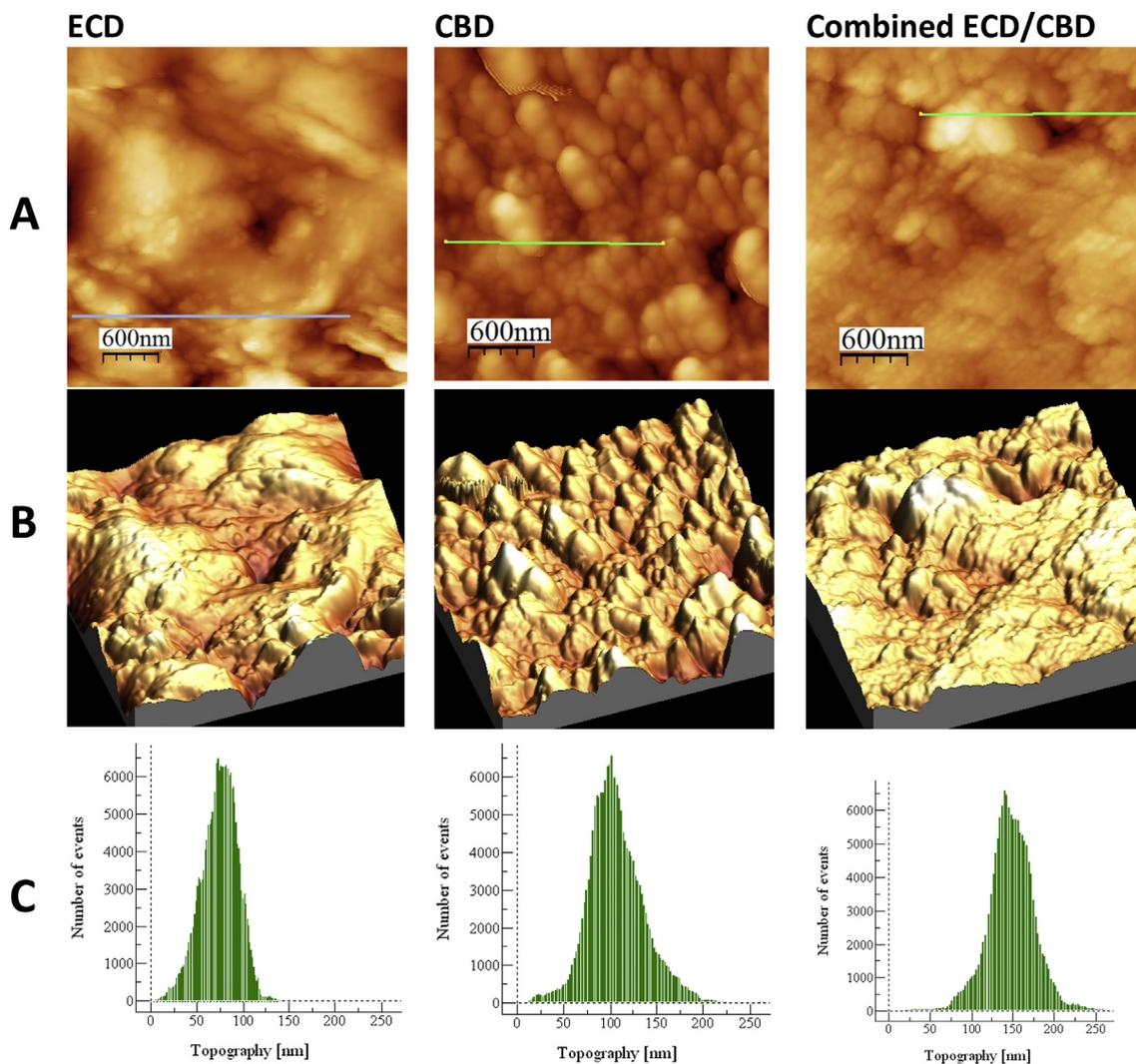
**Fig. 5.** AFM results for different copper selenide films, (a) 2-dimensional micrographs, (b) 3-dimensional micrographs, and (c) surface topographical distribution.
