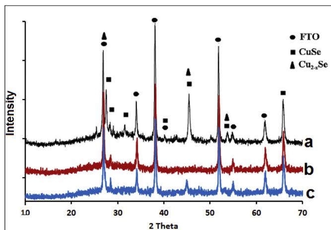
**Fig. 6.** XRD patterns measured for different CuSe film preparations: (a) ECD, (b) CBD and (c) ECD/CBD.
