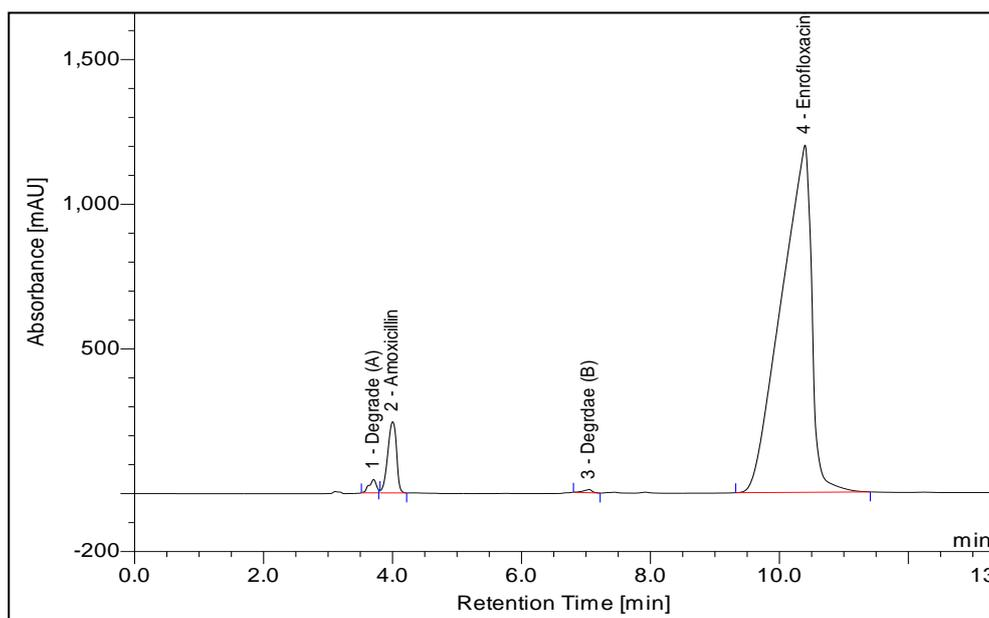
**Figure 2.** Chromatogram of well-separated peaks of the active ingredients (amoxicillin and enrofloxacin) and the degradative materials. Concentration of amoxicillin and enrofloxacin is 0.8 and 0.4 mg/mL, respectively. Degrade A and B are degradants from Amoxicillin.
