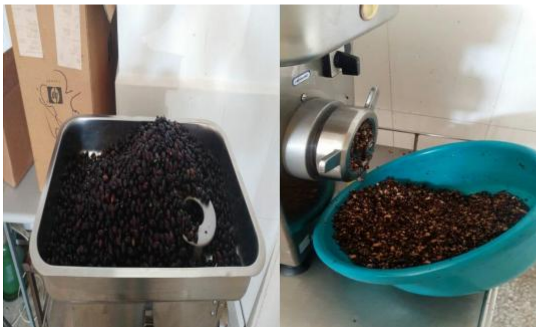
Figure 3. 2 Meat grinding to mill olives
