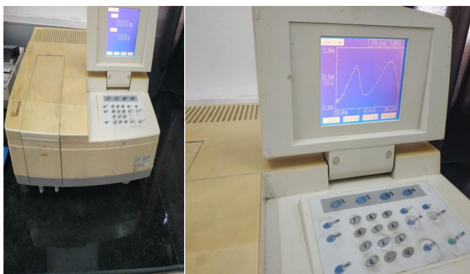
Figure 3. 8 measurement of ultraviolet (K232,K270) by spectrophotometric
