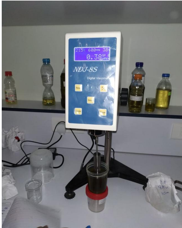
Figure 3. 10 Measurement of viscosity by rotary viscometer.
