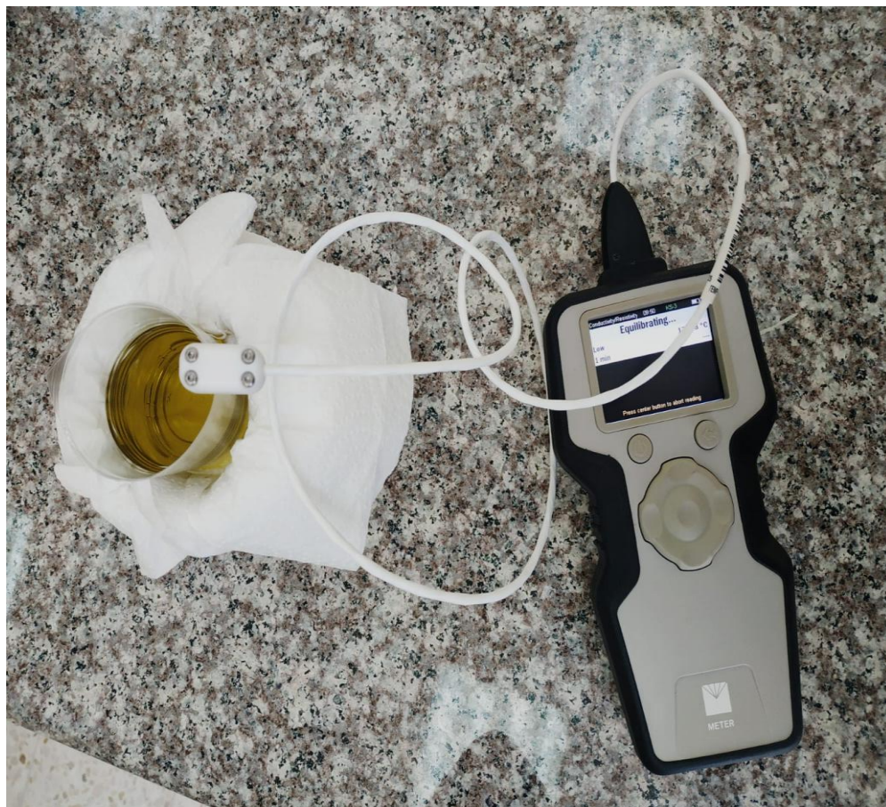
Figure 3. 12 Measurement of thermal conductivity of olive oil .
