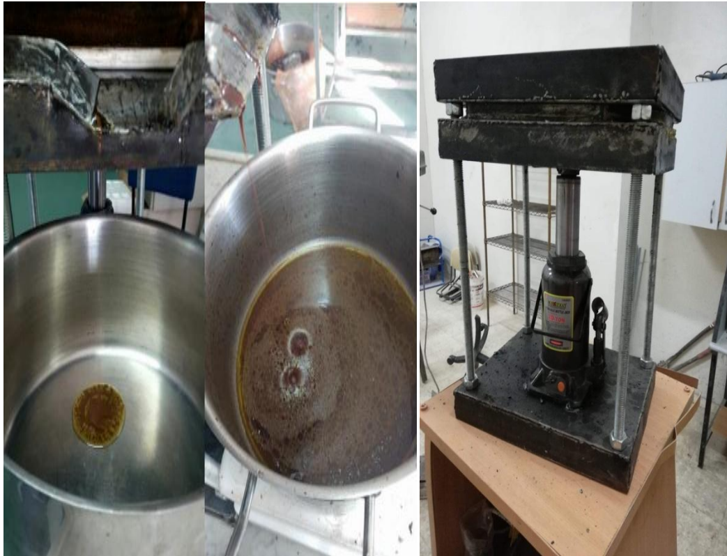
Figure 3. 5 Hydraulic pressure up to 20 ton for separation of liquids.
