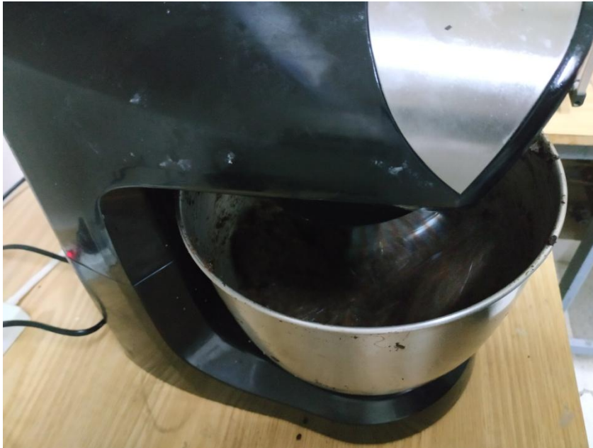
Figure 3. 4 Malaxation process using stainless steel container (mixer).
