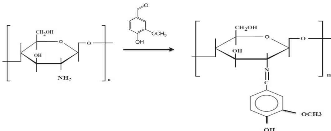
Scheme 1. Preparation of Chitosan-Vanillin Schiff base (polymer I).
