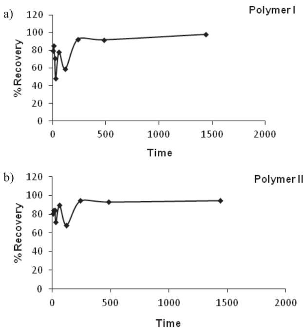
Fig. 7. Effect of contact time on Pb(II) adsorption by: a) polymer I, b) polymer II ( $C_0 = 20$  mg L<sup>-1</sup>,  $T = 30^\circ\text{C}$ ,  $W = 0.05$  g,  $V = 0.05$  L)
