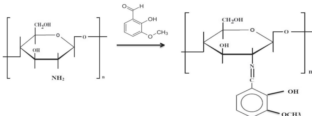
Scheme 2. Preparation of Chitosan-O-vanillin Schiff base (polymer II).
