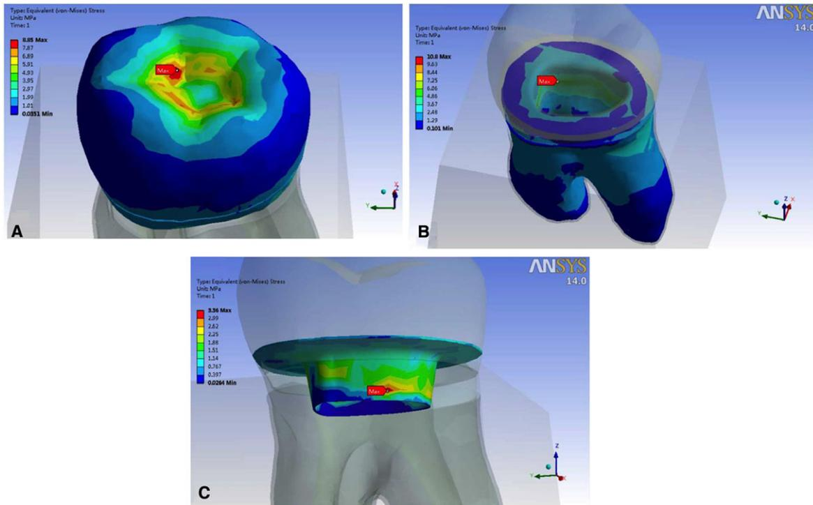
**Figure 4** Distribution of the mvM stresses in molar tooth model B with ceramic endocrown during the masticatory load (MPa). (A) The mvM stresses in ceramic endocrown; (B) the mvM stresses in dentin; (C) the mvM stresses in composite resin luting cement.
