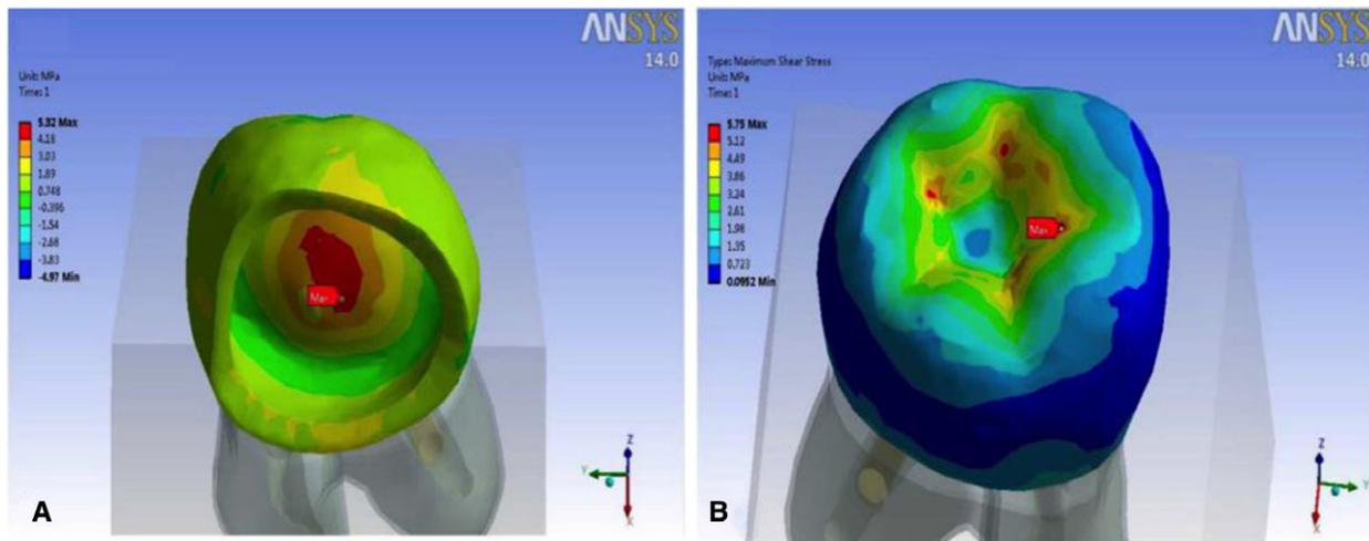
**Figure 7** Distribution of contact stresses in molar tooth model C with FRC posts, composite resin core, and ceramic crown during the masticatory load (MPa). (A) Contact tensile stresses in the ceramic crown; (B) contact shear stresses in the ceramic crown.
