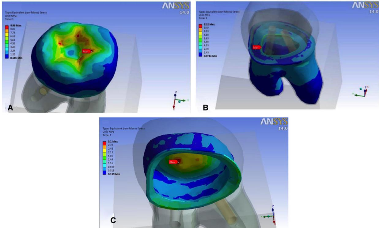
**Figure 6** Distribution of the mvM stresses in molar tooth model C with FRC posts, composite resin core, and ceramic crown during the masticatory load (MPa). (A) The mvM stresses in ceramic crown; (B) the mvM stresses in dentin; (C) the mvM stresses in composite resin luting cement around post.
