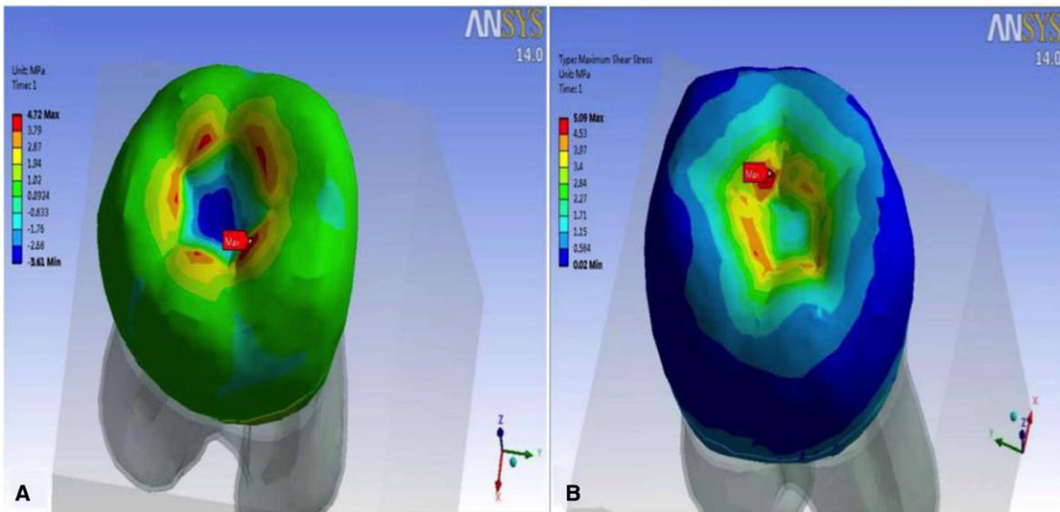
**Figure 5** Distribution of contact stresses in molar tooth model B with ceramic endocrown during the masticatory load (MPa). (A) Contact tensile stresses in the ceramic endocrown; (B) contact shear stresses in the ceramic endocrown.
