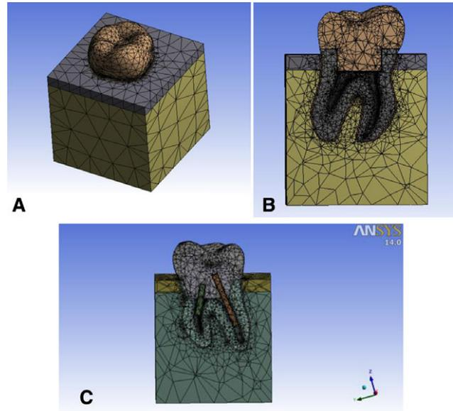
**Figure 2** Meshed models of: (A) intact molar; (B) tooth restored by ceramic endocrown; (C) tooth restored with ceramic crown supported by FRC posts and composite core.
