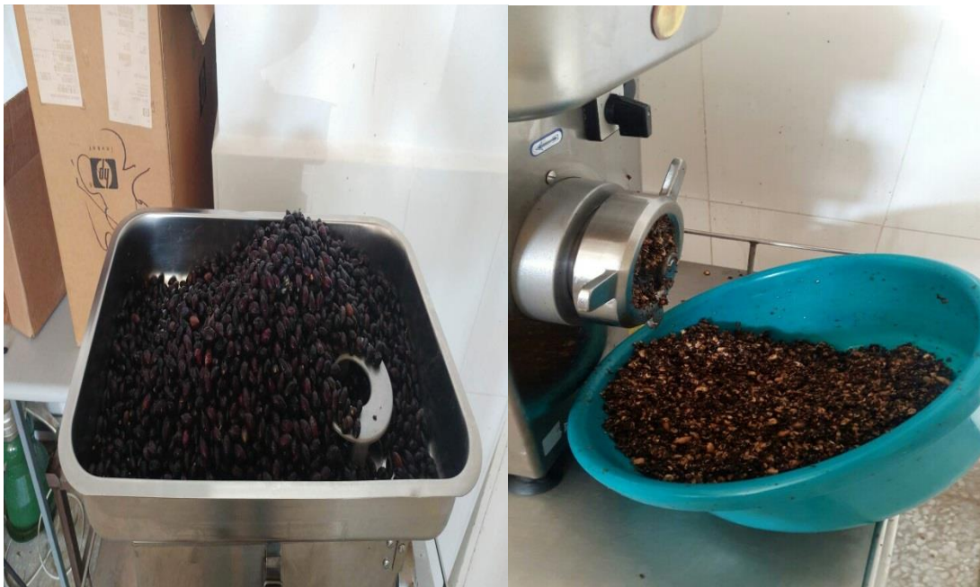
Figure 3.4: Meat grinding to mill olive.
