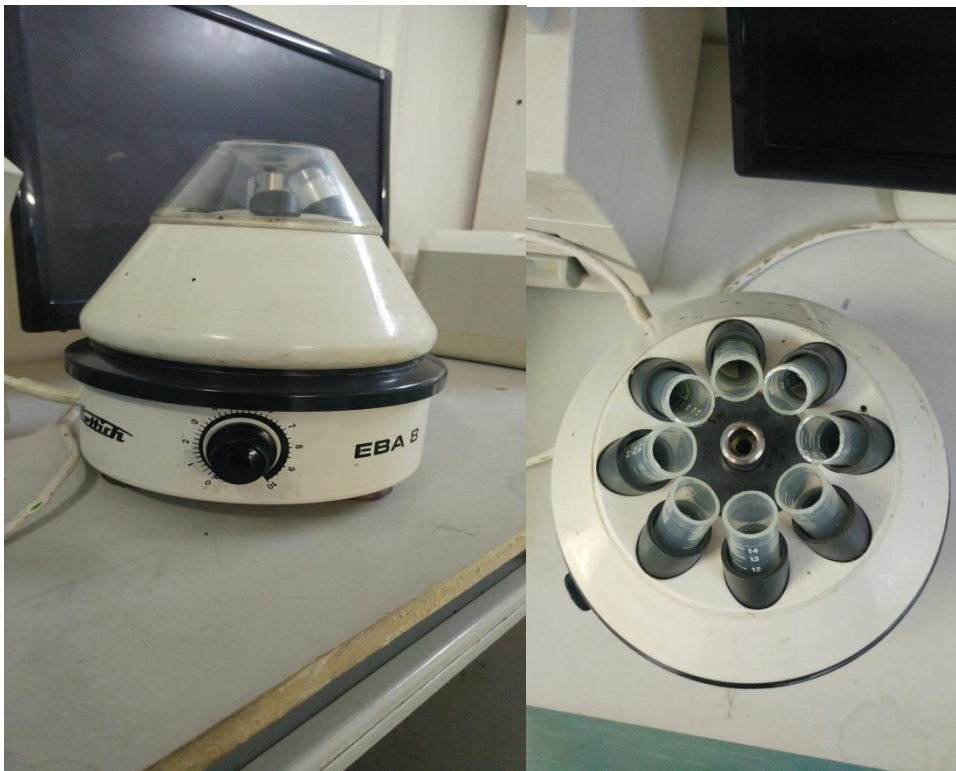
Figure 3.8: The vertical centrifuge (6000 rpm).
