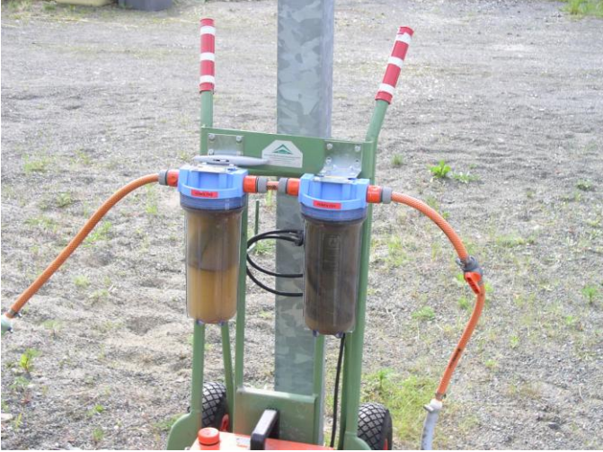
Photo A1: SGR system used as pretreatment stage.
