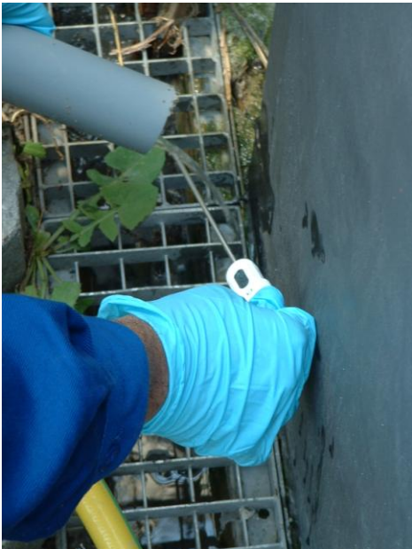
Photo A7: Temperature measured manually from RBC effluent.
