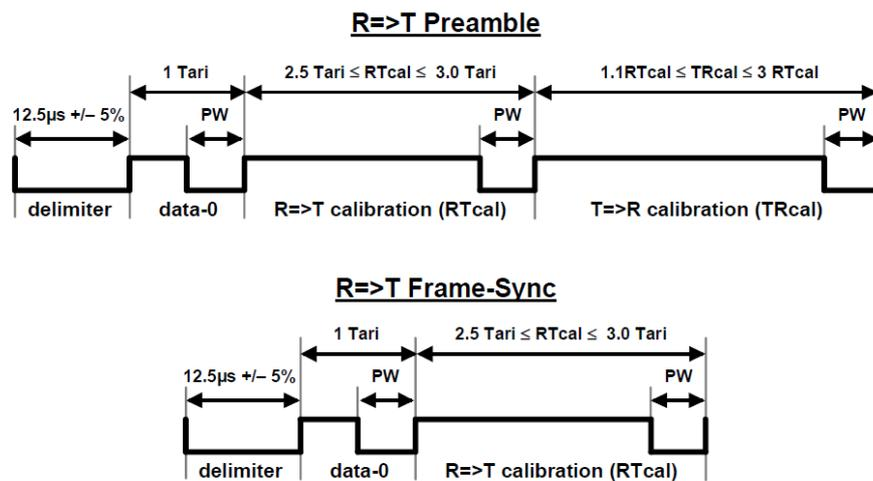
**Figure 2.6:** Reader to tag Preamble and Frame-Sync [2].
