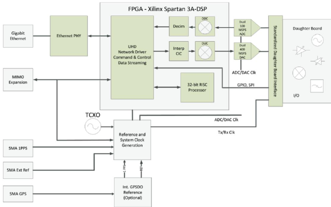
**Figure 3.4:** USRP N210 Hardware Architecture [7].
