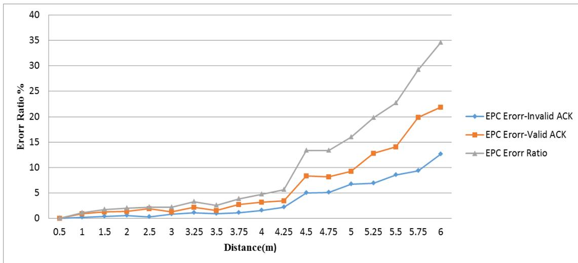
**Figure 4.5:** Error Ratio versus Reading Distance.
