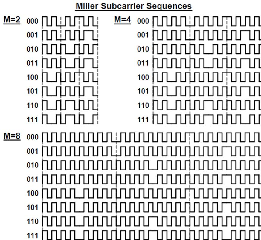
**Figure 2.8:** Illustration of the different miller type data encoding [2].
