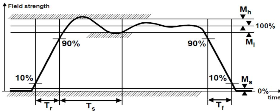
**Figure 2.5:** Reader Power-Up and Power-Down RF Envelop [2].
