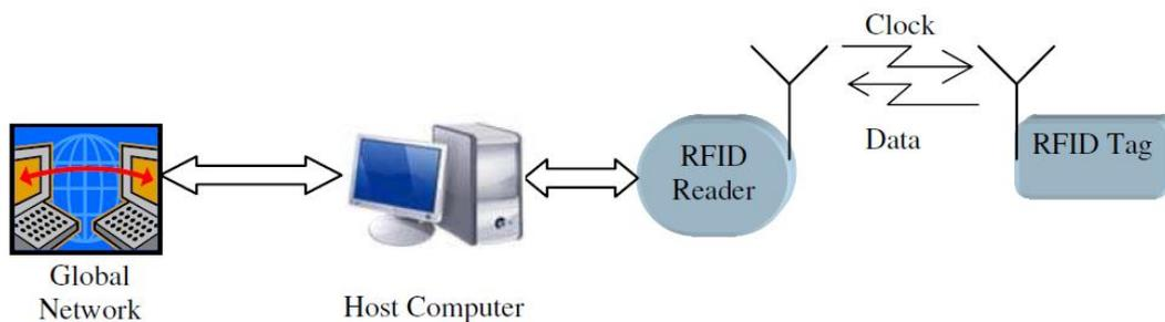
**Figure 2.1:** A block diagram of RFID system [34].
