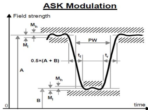
**Figure 2.4:** Reader to Tag RF Envelop [2].
