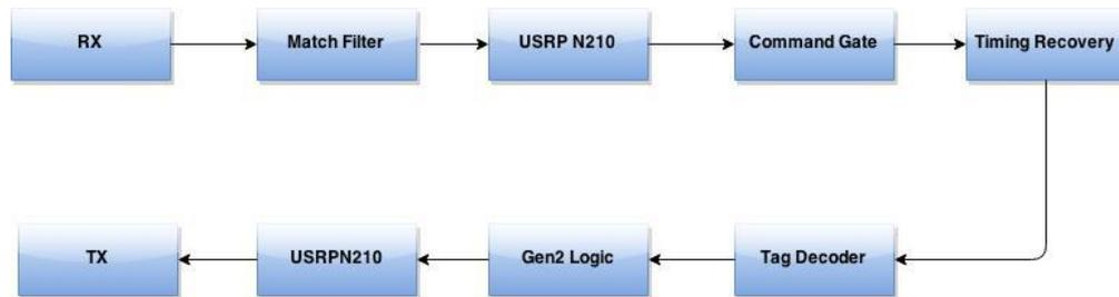
**Figure 3.6:** Gen2 RFID Reader System Architecture.
