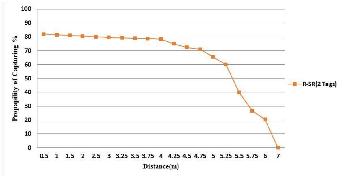
**Figure 4.7:** Probability of Capturing Versus Reading Distance.
