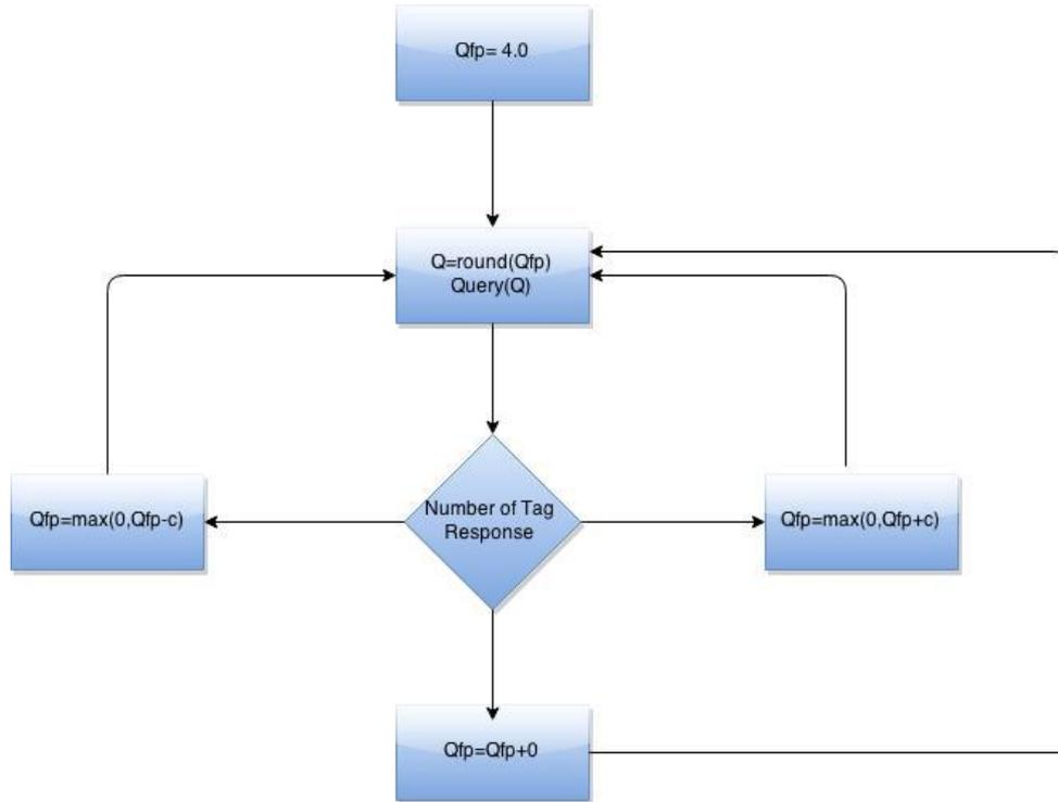
**Figure 2.12:** Q-algorithm used by EPC Gen-2.
