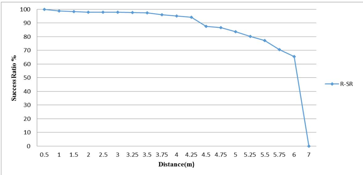
**Figure 4.4:** Success Reading Ratio versus Reading Distance.
