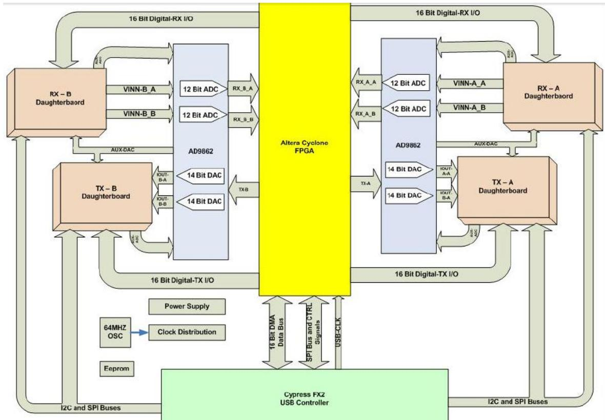
**Figure 3.3:** USRP1 Hardware Architecture [46].
