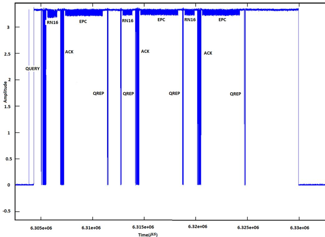
**Figure 4.8:** Communication Cycle between Our Reader and Tags Based on DFSA.
