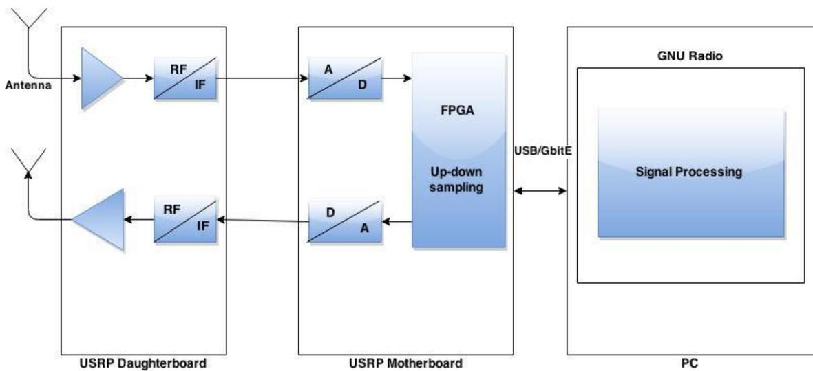
**Figure 3.1:** Software-Defined Radio Block Diagram.
