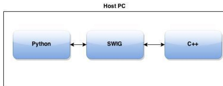
**Figure 3.5:** Software Architecture in GNU Radio.
