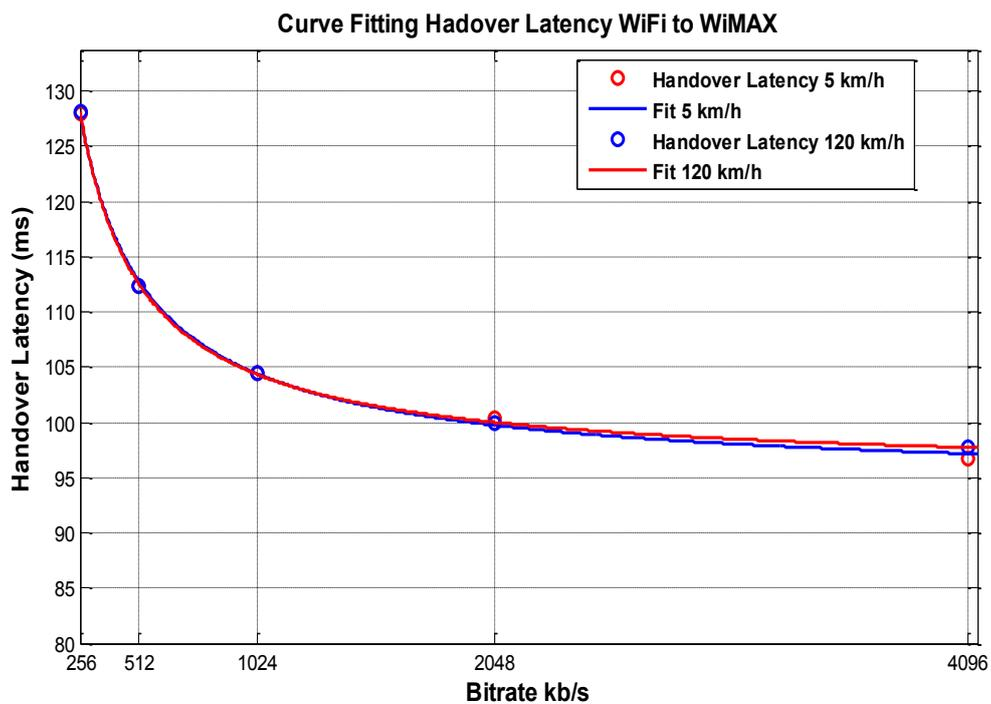
Figure 5.5: Curve Fitting for Handover Latency WiFi to WiMAX
