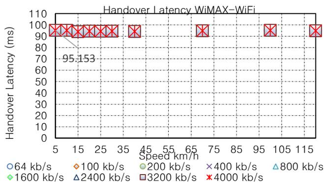
Fig. 13. Handover latency measured between media server and mobile node for different bit rates when the mobile node moves from WiMAX to WiFi.
