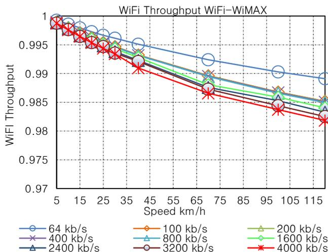
Fig. 2. Normalized throughput measured between media server and WiFi interface on the mobile node for different bit rates in WiFi to WiMAX scenario.
