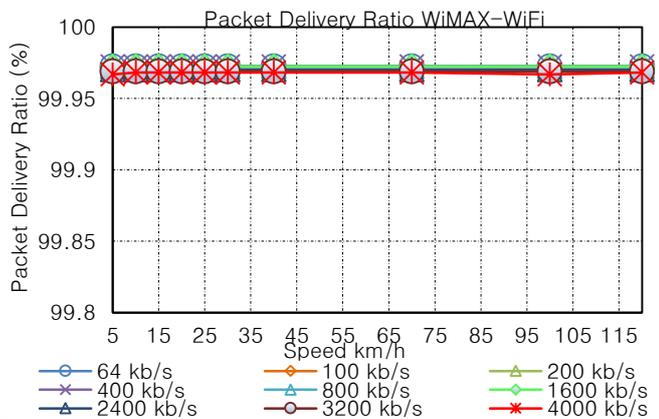
Fig. 15. Total Packet Delivery Ratio for different bit rates when the mobile node moves from WiMAX to WiFi network.
