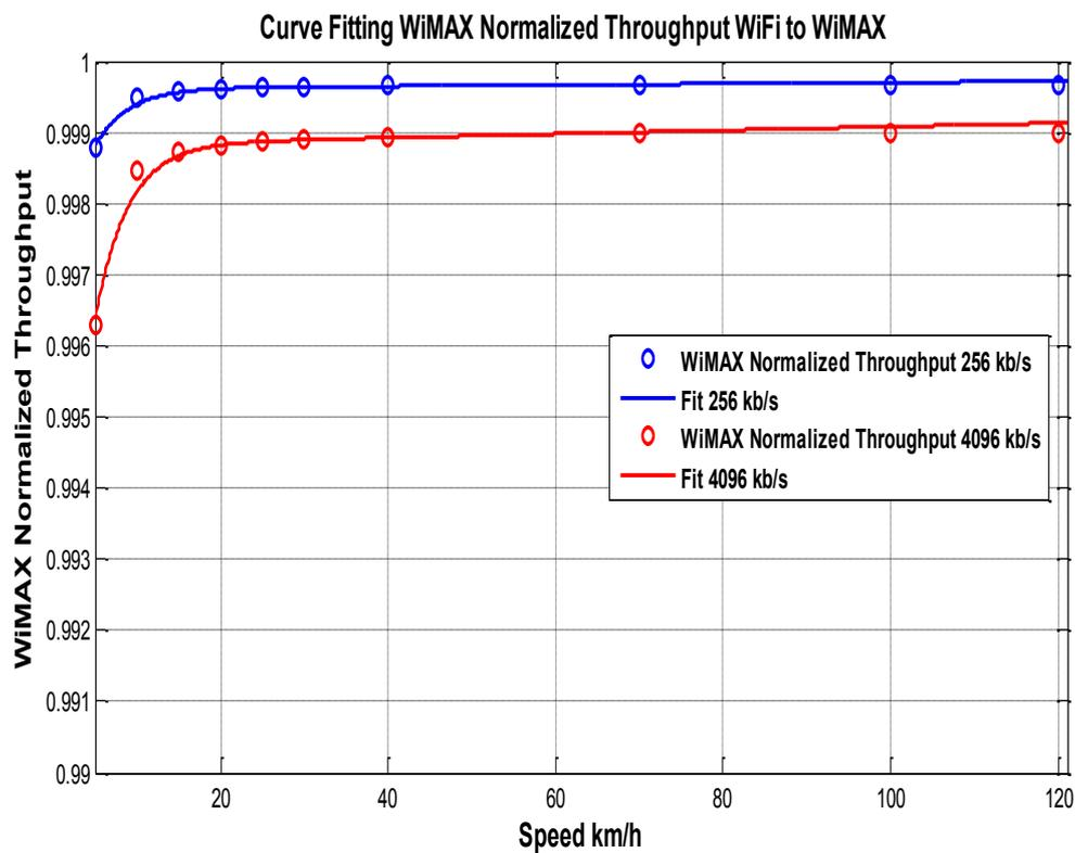
Figure 5.3: Curve Fitting for WiMAX Normalized Throughput WiFi to WiMAX
