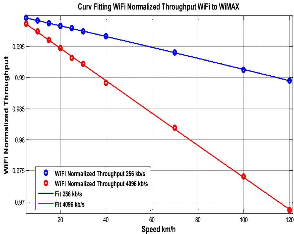
Figure 5.1: Curve Fitting for WiFi Normalized Throughput WiFi to WiMAX
