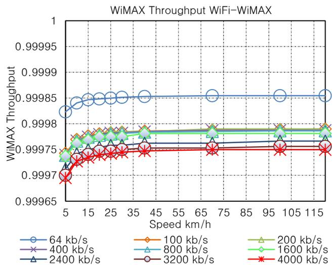
Fig. 3. Normalized throughput measured between media server and WiMAX interface on the mobile node for different bit rates in WiFi to WiMAX scenario.
