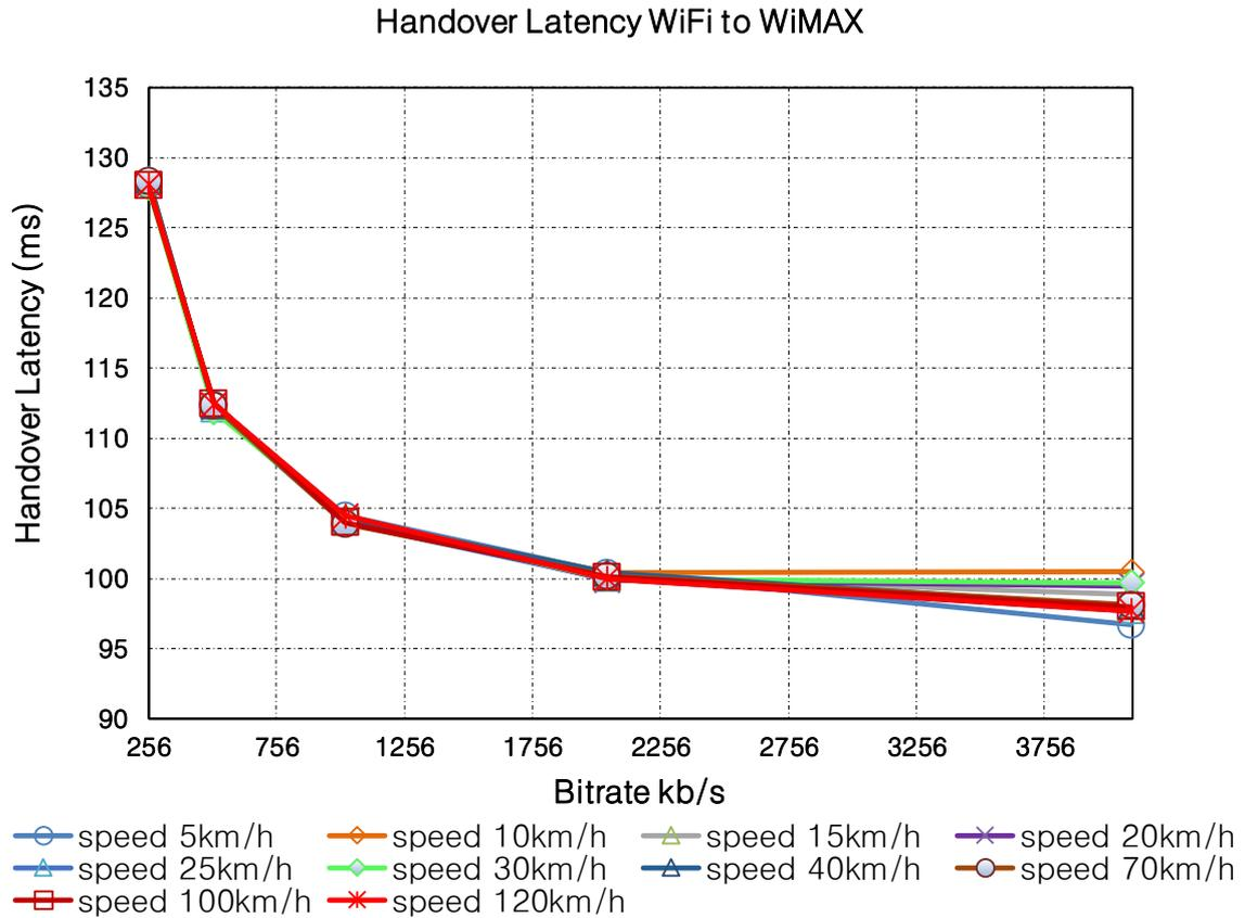
Figure 4.12: Handover Latency as a function of applications bitrate in WiFi to WiMAX scenario.
