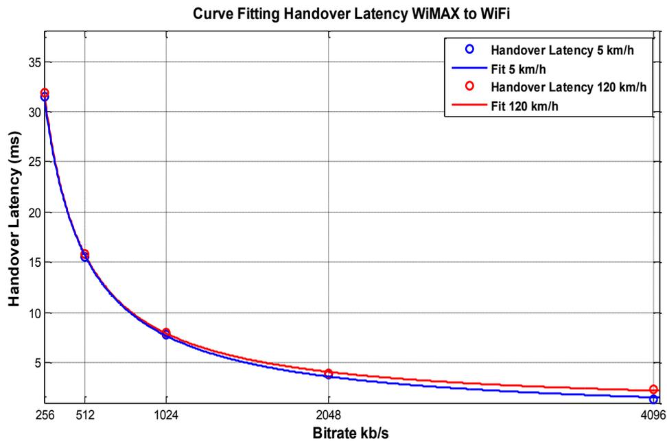
Figure 5.7: Curve Fitting for Handover Latency WiMAX to WiFi
