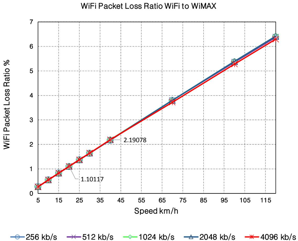
Figure 4.5: WiFi packet loss ratio in WiFi to WiMAX scenario.
