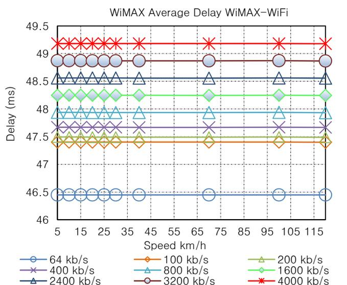
Fig. 8. Average End-to-End Delay measured between media server and WiMAX interface of the mobile node for different bit rates.
