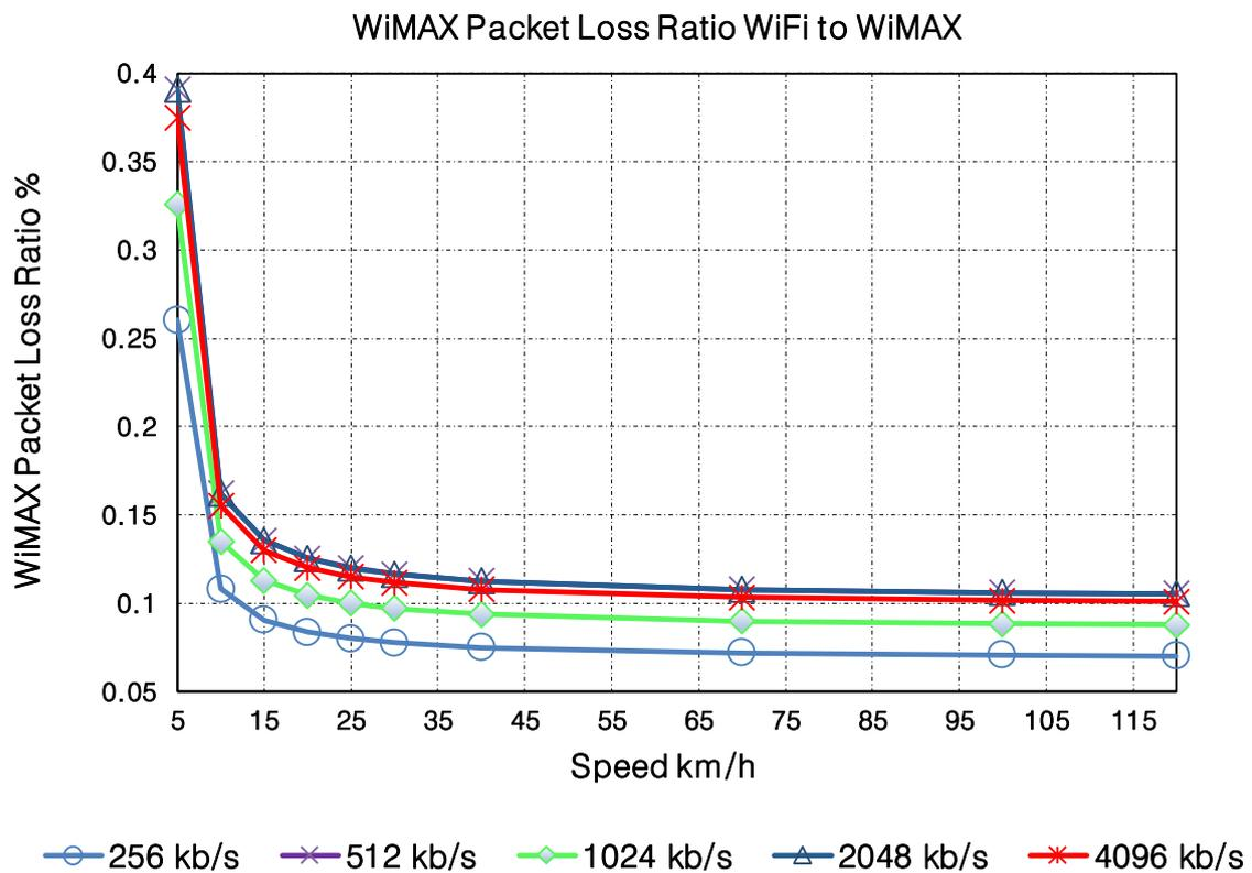
Figure 4.7: WiMAX packet loss ratio in WiFi to WiMAX scenario.
