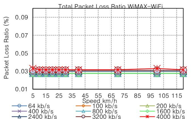
Fig. 11. Total Packet Loss Ratio for different bit rates when the mobile node moves from WiMAX to Wi-Fi network.
