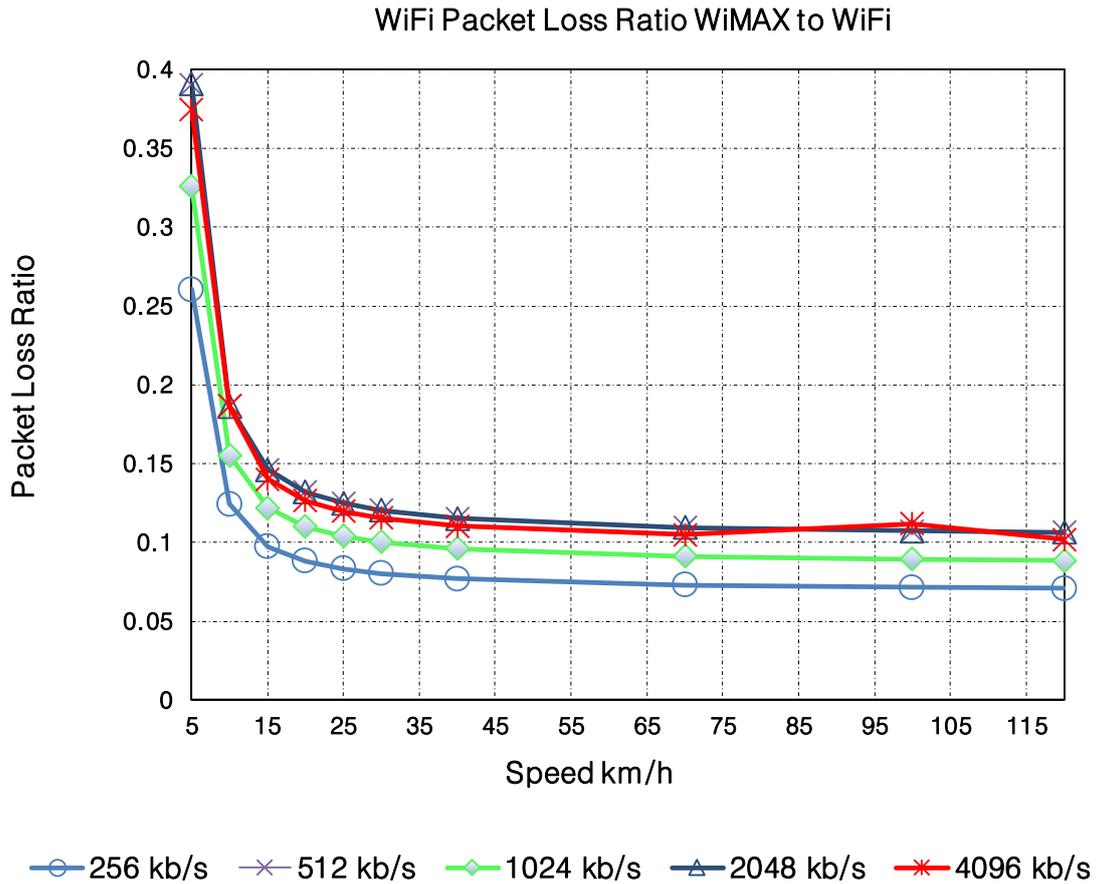
Figure 4.8: WiFi packet loss ratio in WiMAX to WiFi scenario.
