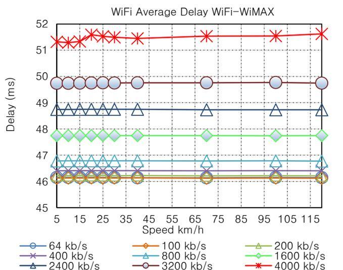
Fig. 6. Average End-to-End Delay measured between media server and Wi-Fi Interface of the mobile node for different bit rates.
