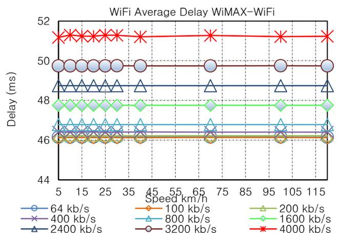
Fig. 9. Average End-to-End Delay measured between media server and WiMAX interface of the mobile node for different bit rates.
