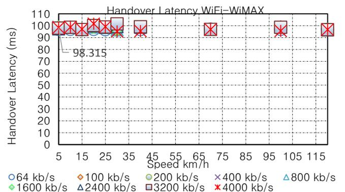
Fig. 12. Handover latency measured between media server and mobile node for different bit rates when the mobile node moves from Wi-Fi to WiMAX.
