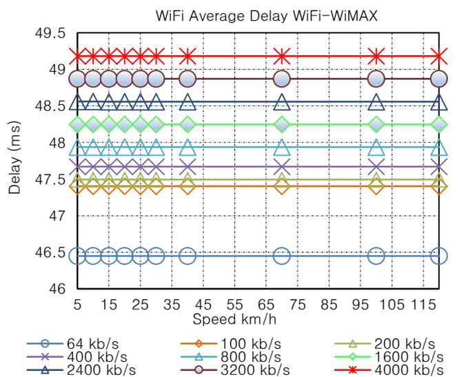
Fig. 7. Average End-to-End Delay measured between media server and Wi-Fi interface of the mobile node for different bit rates.
