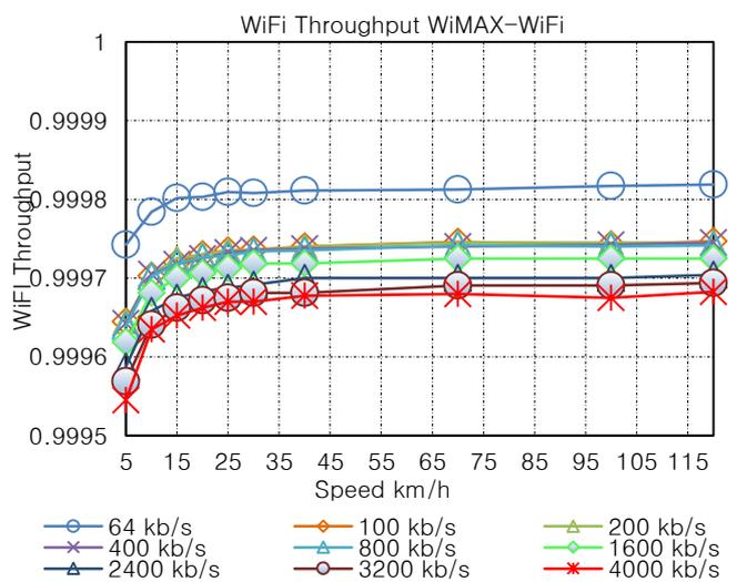
Fig. 5. Normalized throughput measured between media server and WiFi interface on the mobile node for different bit rates in WiMAX to WiFi scenario.
