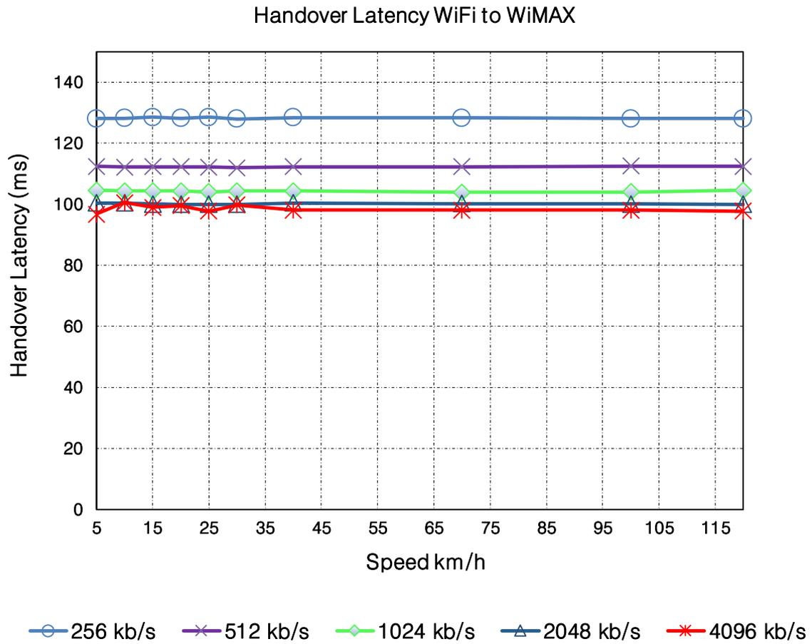
Figure 4.11: Handover Latency as a function of MN speed in WiFi to WiMAX scenario.
