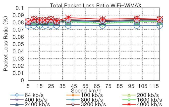
Fig. 10. Total Packet Loss Ratio for different bit rates when the mobile node moves from Wi-Fi to WiMAX network.
