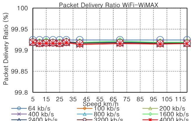
Fig. 14. Total Packet Delivery Ratio for different bit rates when the mobile node moves from Wi-Fi to WiMAX network.
