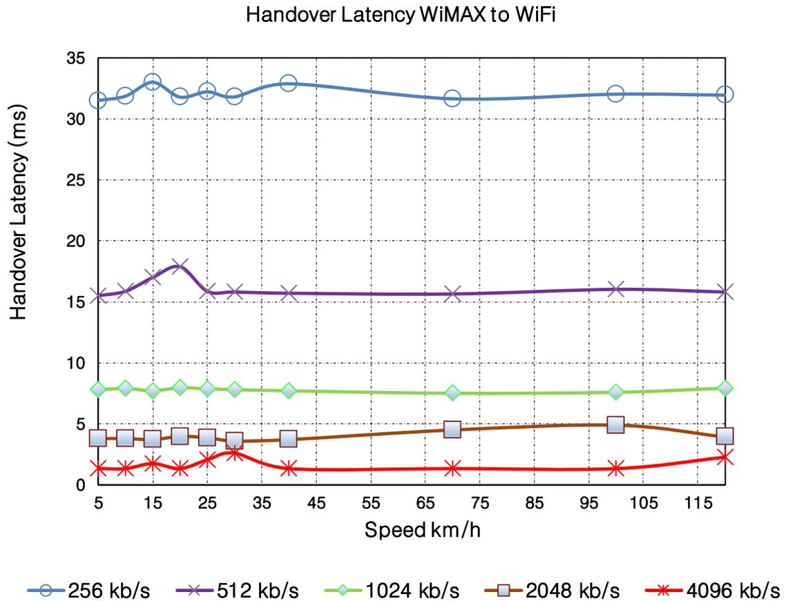
Figure 4.13: Handover Latency as a function of MN speed in WiMAX to WiFi scenario.
