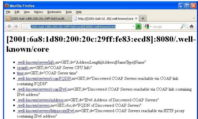
Figure 7. CoRE Link Format rewriting. On top, the result of a CoAP request in CoRE Link Format. Below, the automatically created HTML page.
